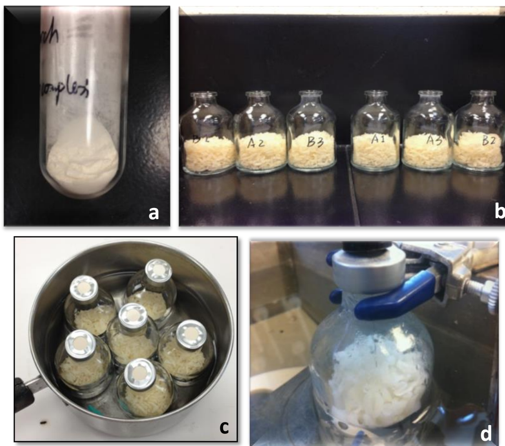
Figure 3.1 (a) 2AP-ZnCl 2 complex was dispersed in dry corn starch, (b) instant rice samples were in 50 mL vials, (c) instant rice samples were heated after sealing with PTFE-lined caps in a boiling water bath, (d) HS-SPME extraction of aroma from cooked rice samples.
