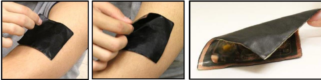
Figure 5.15. The actuation system circuit in stretched and twisted views to demonstrate the stretchability and flexibility.
