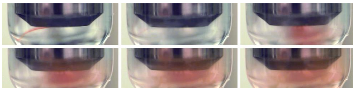
Figure 4.2 Mixing pattern of solution (red, flowing from the tapped ultrasonic horn) and antisolvent (white, flowing from the lower right) within the spray sonocrystallization rig. The second frame marks the start of sonication. Frames were extracted from video every 33 ms.
