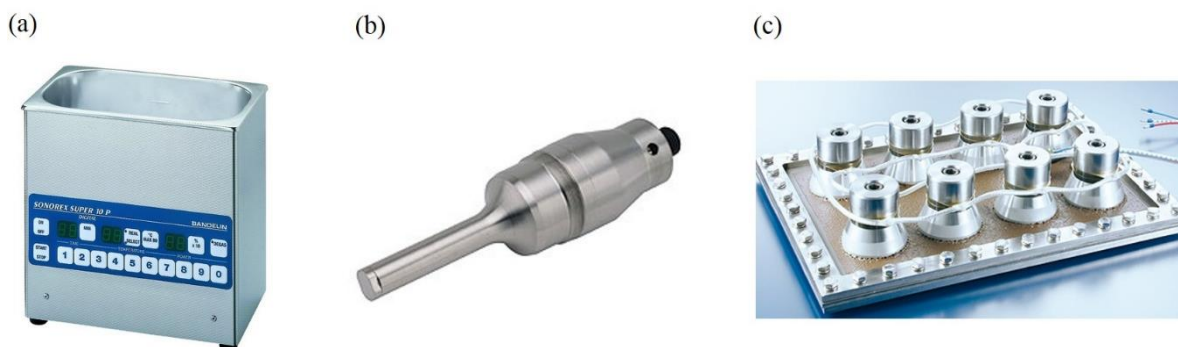
Figure 1.20 Different types of ultrasound generators: (a) ultrasonic bath, 74 (b) ultrasonic horn, 75 and (c) ultrasonic plate transducer. 76
