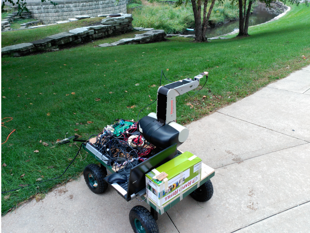
Figure 3.2: An operator pulls and pushes the cart continuously in a straight line through a sloped and bumpy grass field about 8 meters long. In the image the sloped terrain and the cart are visible.
