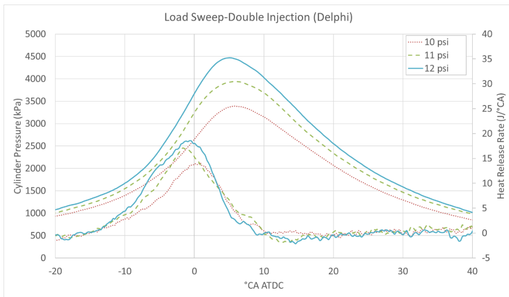
Figure 6.72 Pressure and HRR curves – Delphi – Intake pressure sweep (double inj.)
