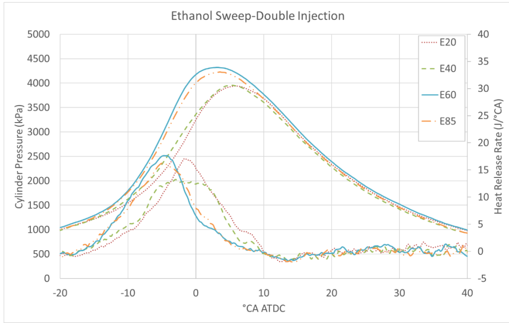
Figure 6.32 Pressure and HRR curves for various fuel blends (double injection)
