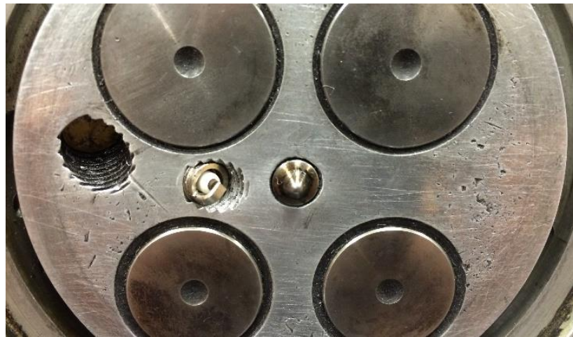
Figure 6.10 Spark plug installed in cylinder head
