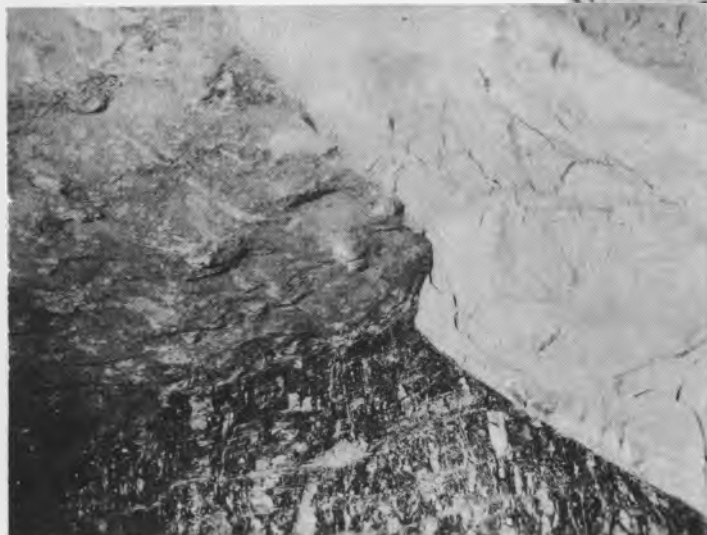
Fig. 4. - South side of south "cut-out" on west side of 4th NW back entry. The dark material at the upper left is limestone, that in the extreme upper right corner is silty shale, and the light colored material is coarse-grained sandstone. Note the smoothness of the contact of the coal and sandstone at the coal-limestone contact.
