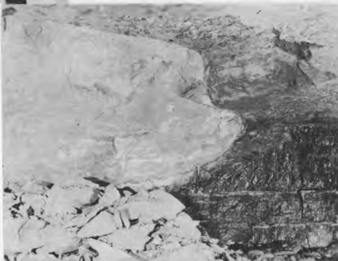
Fig. 3. - East side of "island" of coal off 4th NW entry. Here the fill material consists almost entirely of silty shale. The light streaks are clay.
