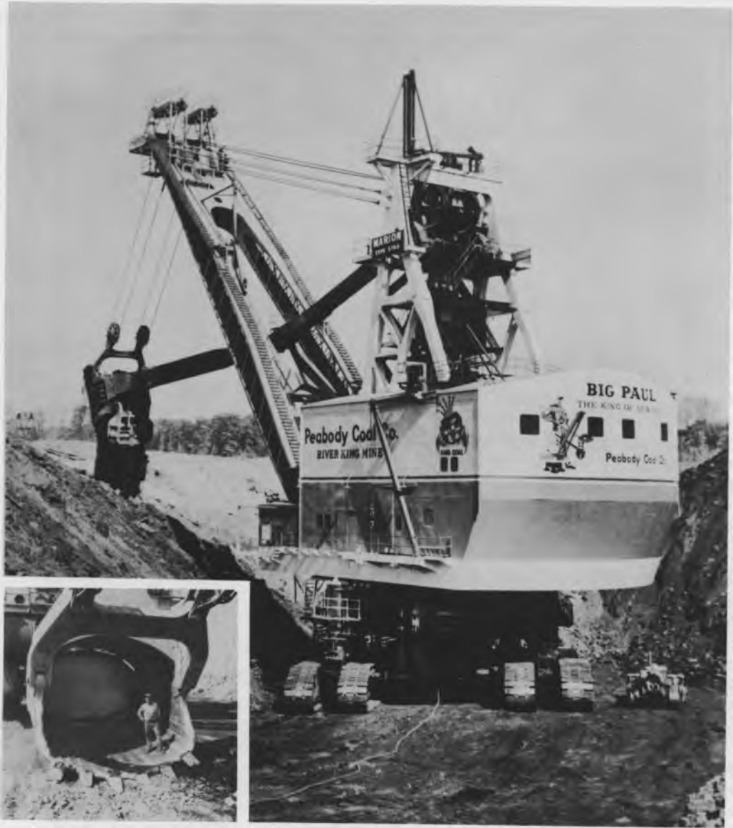
Stripping shovel of 70 cubic yard capacity removing overburden from No. 6 Coal near Freeburg, St. Clair County. Courtesy of Peabody Coal Company.
