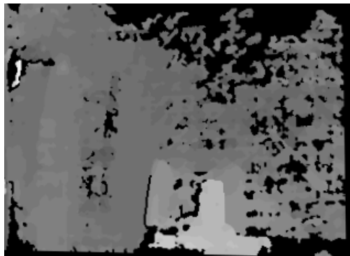
Figure 11: Disparity image using disparity as grayscale value
