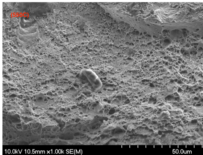
Figure 5.3: SEM 1000 times magnification of post-tensile samples under RT, 450°C and 550°C. RT sample was featured by cracks and cleavages, while 450°C and 550°C samples displayed more holes, voids and dimples.
