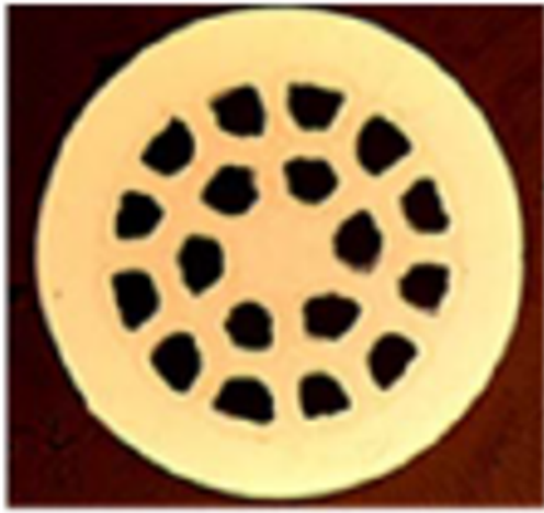
Figure 2.8: An example wire cross section, showing darker \text{MgB}_2 filaments embedded in a copper matrix [20]
