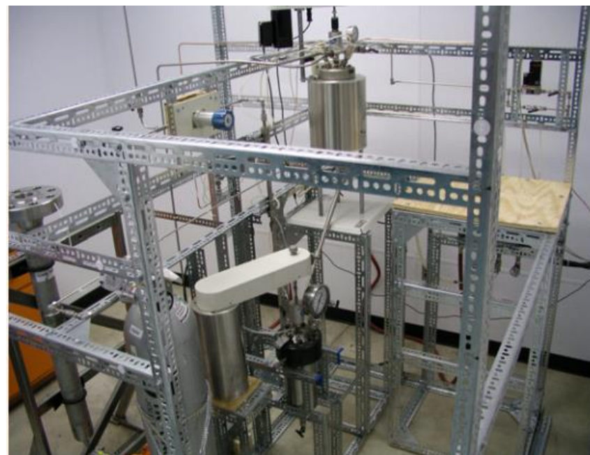
Figure 2-7. UIUC HTL Laboratory continuous reactor system: (a) schematic of the continuous hydrothermal process (CHTP) reactor system, and (b) photo of the CHTP reactor system setup (Ocfemia et al., 2006a; Ocfemia et al., 2006b)
