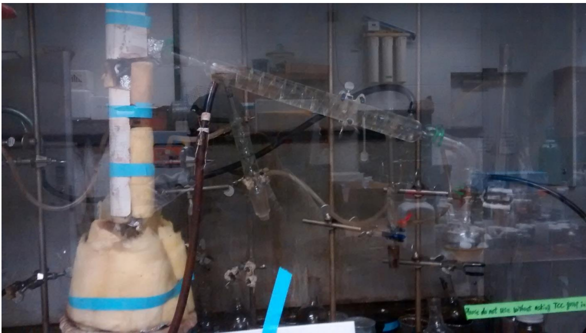
Figure L-1. Basic set-up of a simple distillation system (a) cartoon illustration (b) actual set-up
