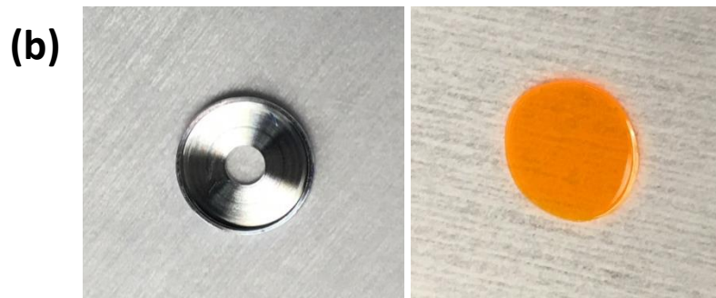
Figure 5.3 (cont.) (a) 3D schematic of the large scale pixel module. (b) Photograph of custom-made aluminum cap and QD-polymer slab.
