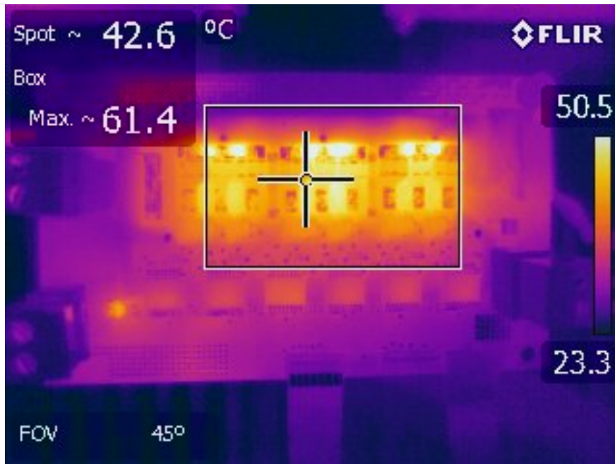
Figure 5.11: Hard-switched, 30 V to 300 V conversion. P_{in} = 106 W, P_{out} = 100 W, f_{sw} = 72 kHz, L = 22 \mu H.
