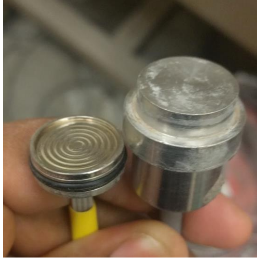
Figure 5 Pressure sensors: 0 – 15 psi (left), 0 – 100 psi (right)
