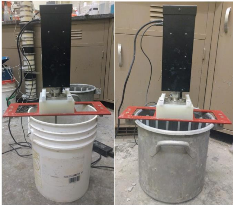
Figure 42 Rheology test setup used: 5 gallon bucket (left), ICAR container (right)
