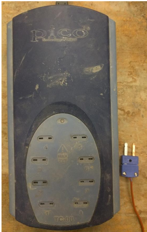
Figure 8 Data Logger (on left) and type T thermocouple (on right)
