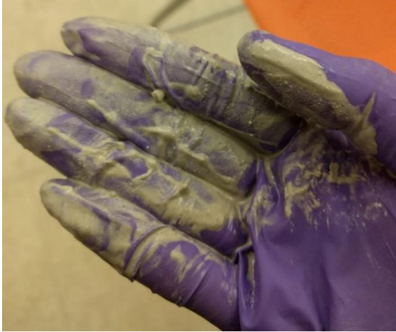
Figure 17 Fines found at the bottom of the bucket after soaking the sieved aggregate in water for a week
