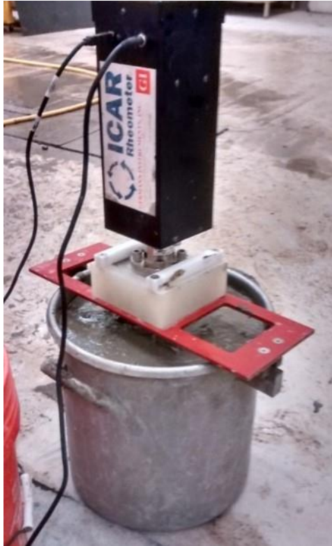
Figure 7 ICAR rheometer test setup
