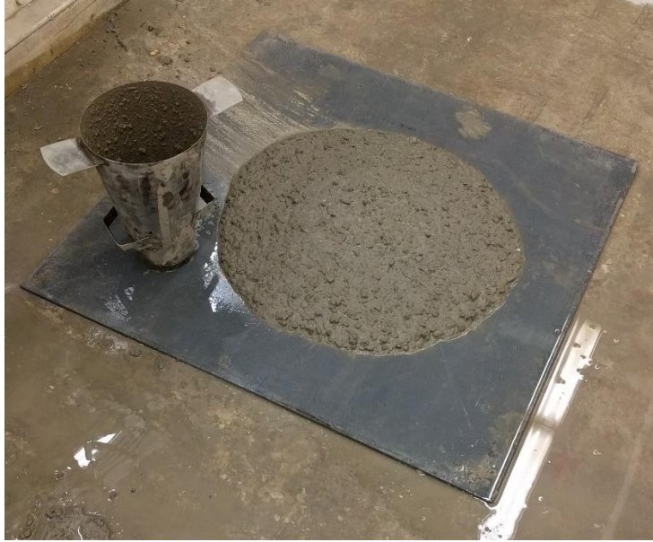
Figure 2 Slump flow test
