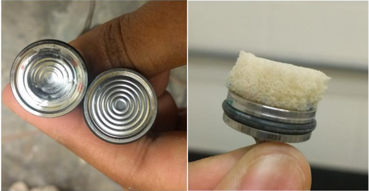
Figure 52 Damage of the sensor (left) due to impingement of the aggregates and sponge added (right)
