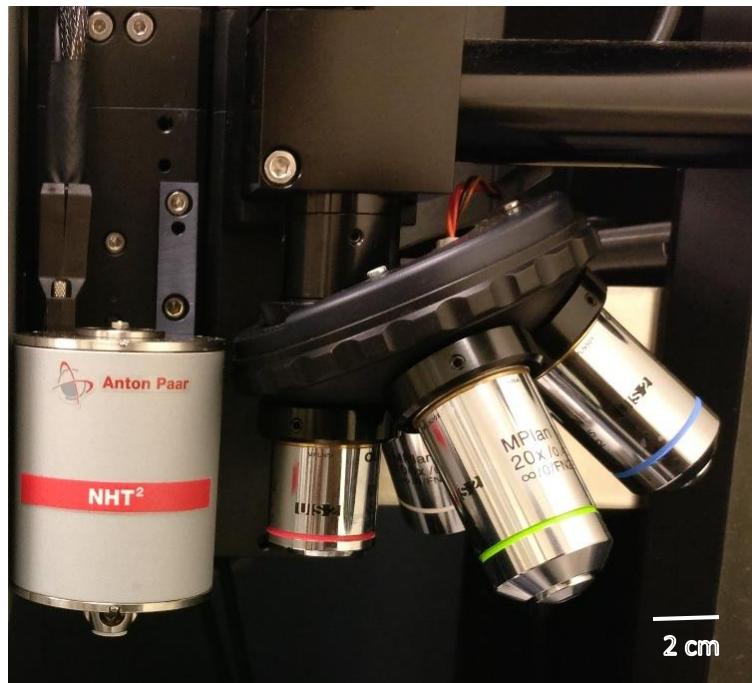
Figure 7.6 Anton Paar Nanoindentation Tester head and the integrated Optical microscope (Credits: Kavya Mendu, UIUC, 2017).
