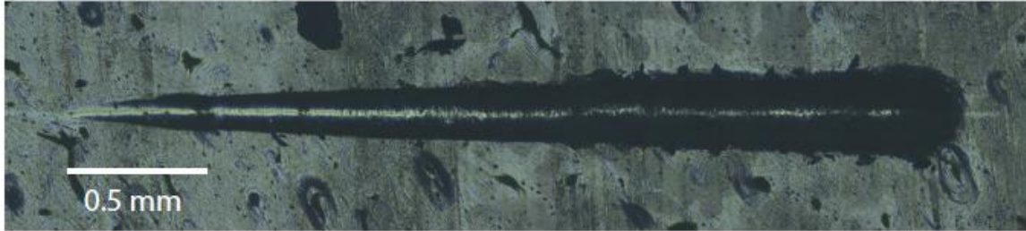
Figure 6.24 Panorama of the scratch test on the transverse (SL) bovine cortical bone specimen. The scratch groove is 3mm long and loading rate is 60 N/min.
