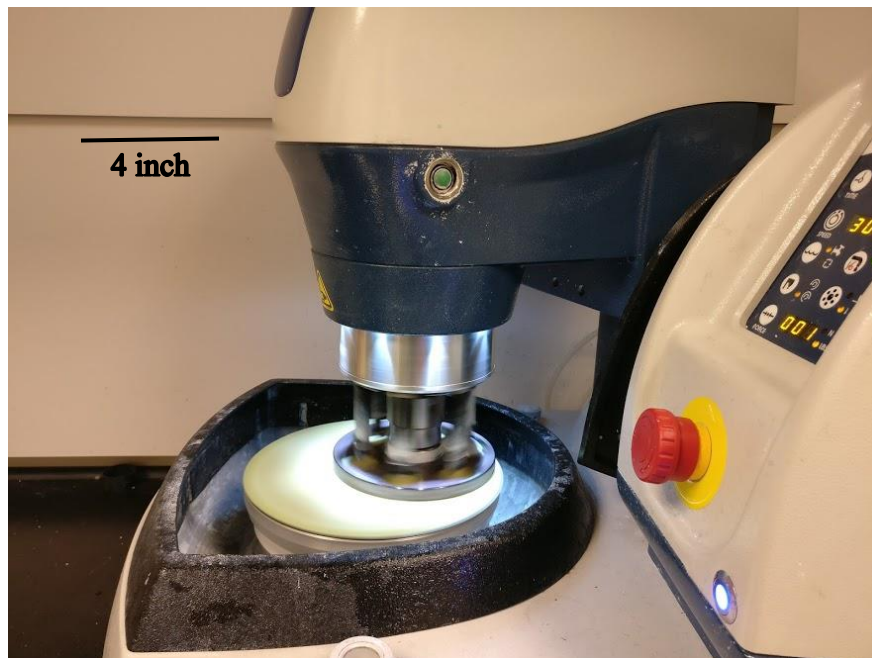
Figure 8.2 Buehler Ecomet 250 Grinder and Polisher, Buehler, Lakebuff, IL. (Credits: Kavya Mendu, UIUC, 2017).
