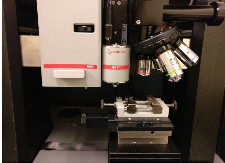
Figure 5.12 Image showing the sample stage, optical microscopy setup, micro scratch tester head and nano indentation tester head (Credits: Kavya Mendu, UIUC, 2017).
