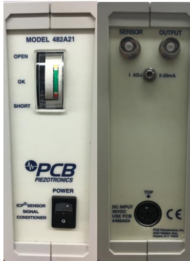
Figure 1.6 Front and Back Panels of the ICP Amplifier and Signal Conditioner for PCB Piezoelectric Pressure Sensors
