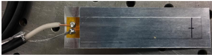
Figure 1.7 Soldered MN4-50-EK Manganin Gauge (Sensing Element Marked with a Cross)
