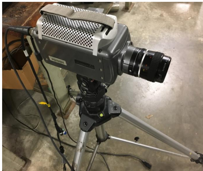
Figure 1.14 Setup for Phantom v5.2 High Speed Camera with a 55 mm Lens
