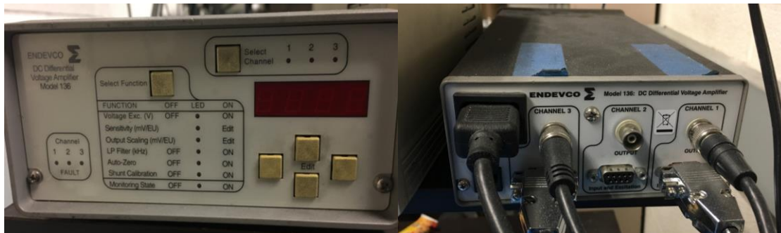
Figure 1.3 Front and Back Panels of the Endevco 136 Amplifier and Signal Conditioner for Kulite Piezoresistive Sensors
