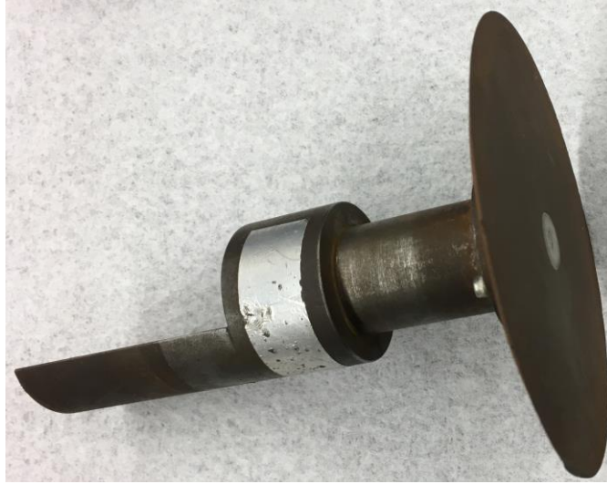
Figure 3.14 Assembled Containment Structure for Kulite XTEL Piezoresistive Sensor
