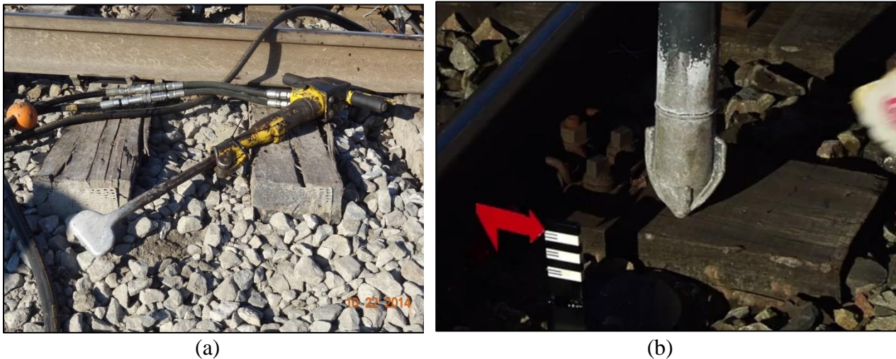
Figure 6.14: Photographs of (a) typical pneumatic tamping head and (b) alternative pneumatic tamping head (courtesy of Robel Company).
