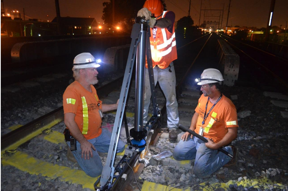
Figure 3.17: Photo of load-frame used to calibrate strain gauges and MDDs on Amtrak NEC by Marty Perkins and Carl Walker (photo courtesy of Deb Mishra).
