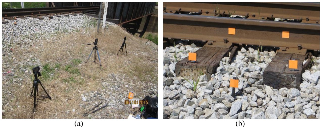
Figure 4.1: Photographs of (a) consumer high-speed video cameras and (b) orange targets attached to rail, timber tie, and stake locations.
