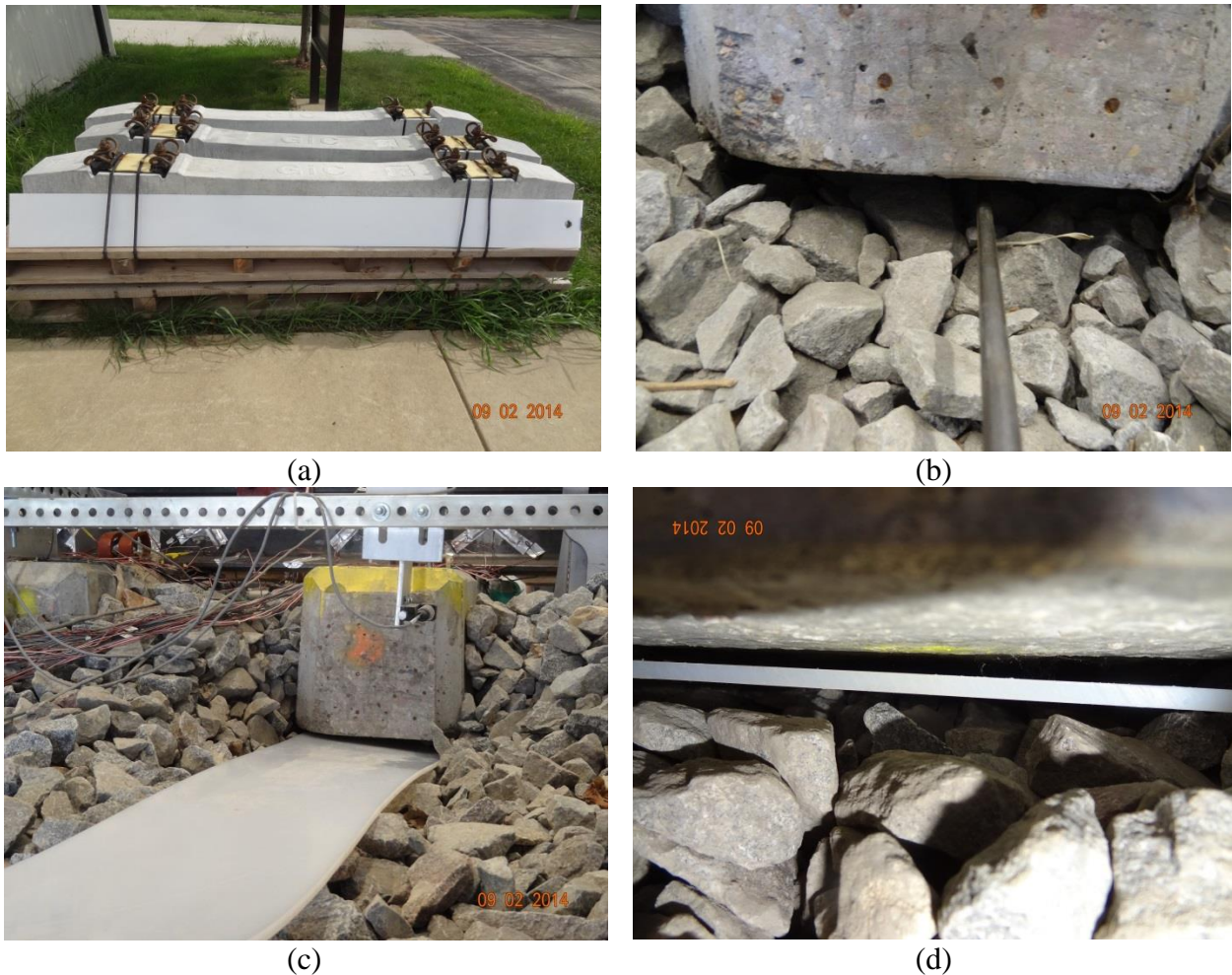
Figure 6.17: Photographs of (a) plastic shims, (b) insertion of metal rod underneath tie, (c) insertion of plastic shim under concrete tie, and (d) shim fully inserted underneath tie.
