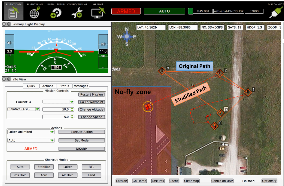
Figure 6.17: Attacker disables the geo-fence and modifies Waypoint 3 so that the drone flies into a no-fly zone. Such a safety-critical function can be protected by running in the SCE.
