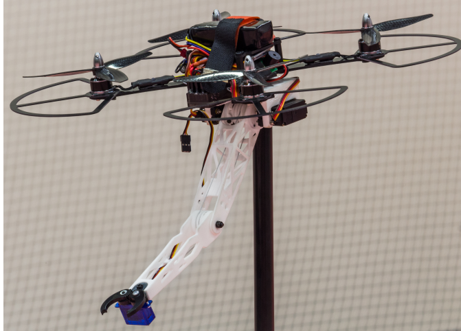
Figure 1.1: Autonomous Quadrotor with 2 DOF Manipulator Arm
