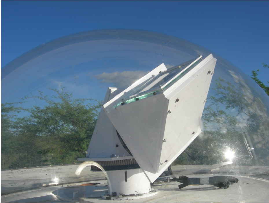
Figure 2.2: The SkyScanner, comprising two independently controlled mirrors to steer the line of sight. Adapted from Fisher [2013].
