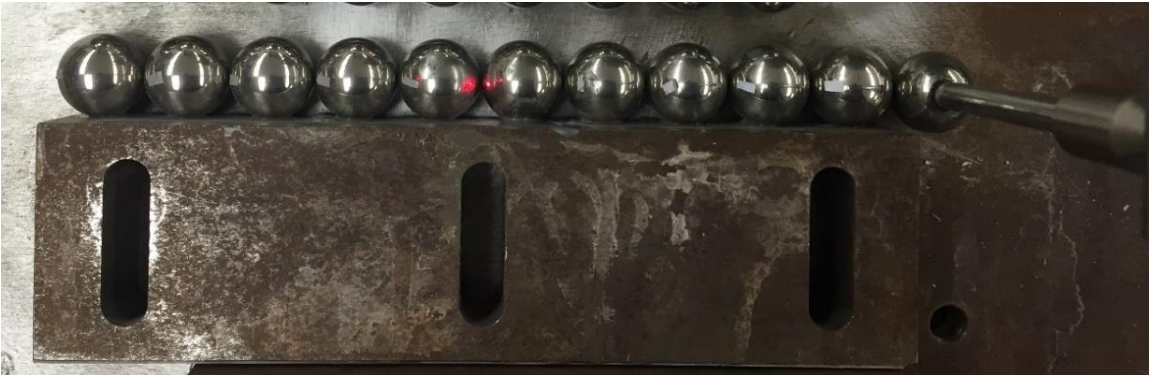
Figure 5.23. Top view of the experimental setup I for the impulsively excited granular chain.
