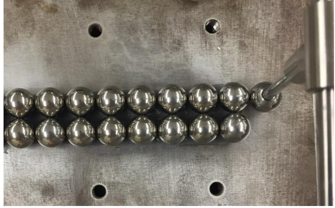
Figure 5.25. Schematic and top view of experimental fixture for the network of coupled granular chains.
