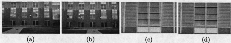
Fig. 6. Pixel-wise accurate registration via matrix rank minimization. (a) and (b): The first and last frames of a batch. (c): Superposition of the blue window labeled in (a) using frame (a) and (b), according to the homographies estimated by our RANSAC-based plane detection and tracking algorithm. (d): Superposition of the same window according to the homographies refined by RASL. The improvement is clear.
