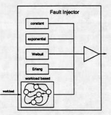
Figure 2: The Fault Injector Object.
