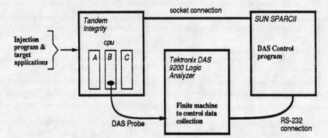
Figure 11: An injection environment using hybrid monitoring.
