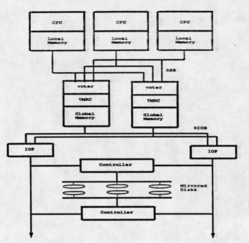
Figure 8: The Tandem Integrity processing subsystem
