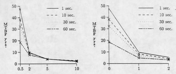
Global Mem. Re-integration (min.) Percent Correlation, Global Mem. Reint (0.5min) Figure 21: System reliability for various subsystem re-integration times.
