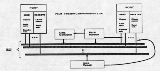
Figure 4: The Fault-Tolerant Communication Link.
