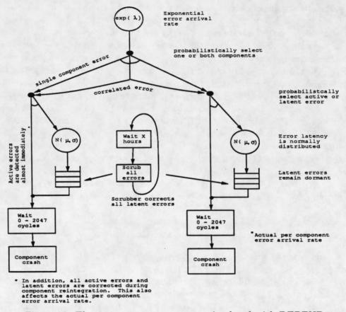
Figure 10: The error occurrence process simulated with DEPEND.
