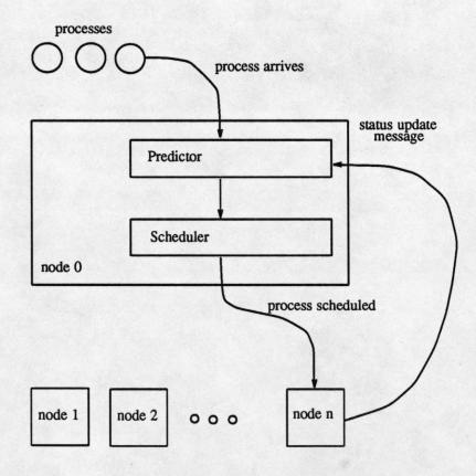
Figure 2. MINQ: Centralized load-sharing with prediction.
