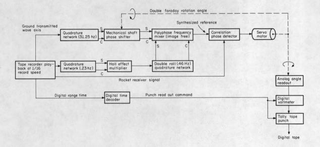
Figure 3. Block diagram of Faraday Rotation Data Processor.
