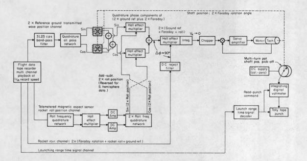
Figure 4. Block diagram of Faraday Rotation Data Processor - more detailed.
