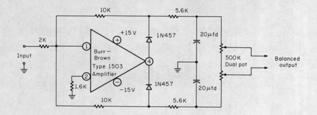
Figure 2. Rectifier filter schematic diagram.
