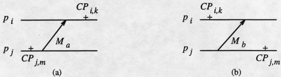
Figure 3: Checkpoint consistency (a) orphan message M_a ; (b) in-transit message M_b .
