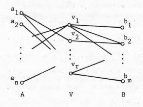
Figure 1. General scheme of a 2-stage connection.
