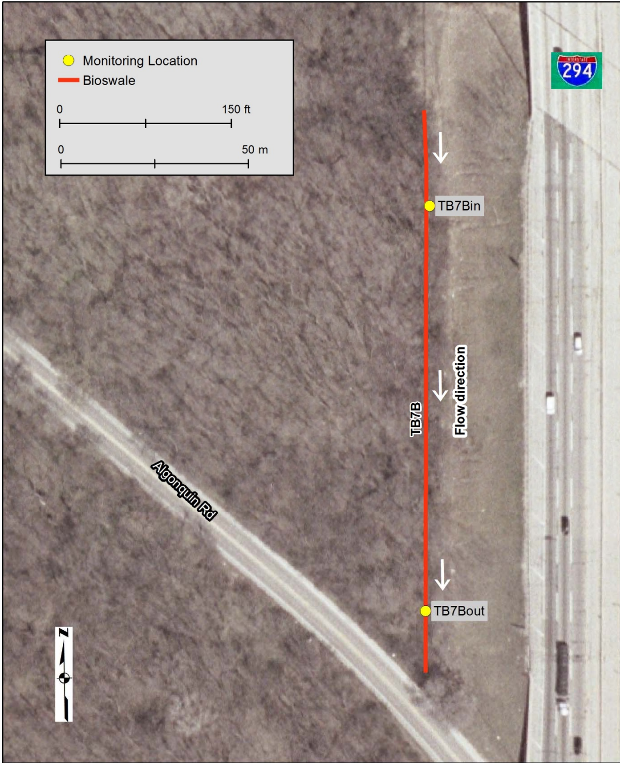
Figure 3. Location of bioswale and monitoring points at TB7B.
