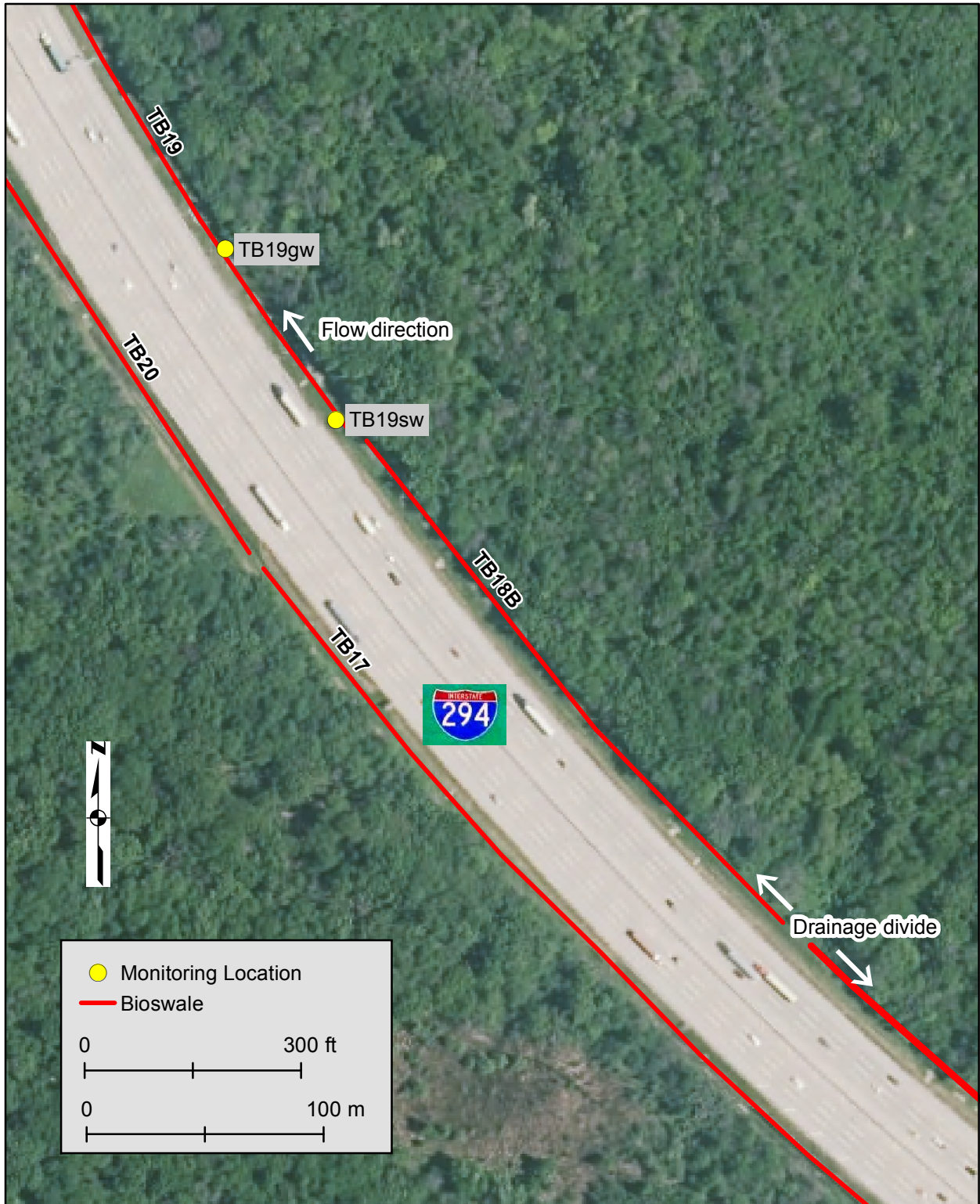
Figure 9. Location of bioswales and monitoring points at TB19.
