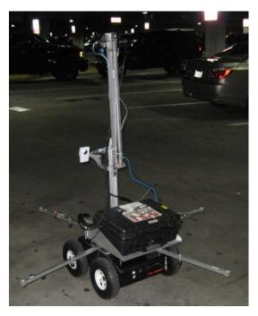
Figure 8. Robotic Roadway Lighting Mobile Measurement System (RRLMMS).
