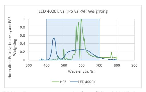
Figure 3. PAR weighting curve versus normalized typical HPS and 4000K LED spectrum.
