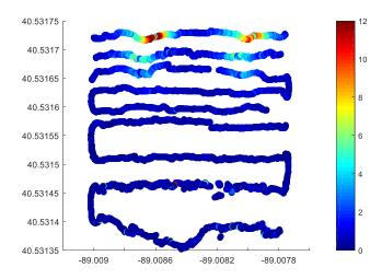
Figure 12. Horizontal illuminance for Normal1 before digital filtering. The horizontal illuminance is represented by the color. The y and x axes are latitude and longitude in degrees.
