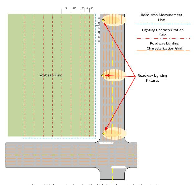
Figure 9. Schematic showing the lighting characterization strategy.
