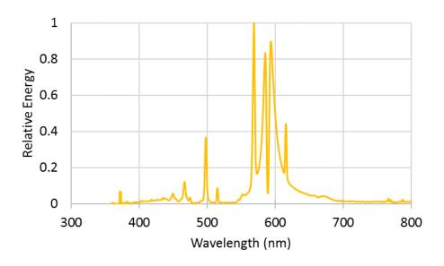
Figure 2. Spectral power distribution of a 2700 K HPS lamp used for lighting roadways.
