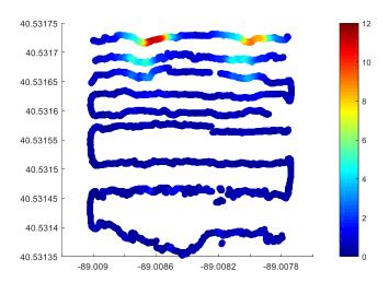
Figure 13. Horizontal illuminance for Normal1 after digital filtering. The horizontal illuminance is represented by the color. The y and x axes are latitude and longitude in degrees.
