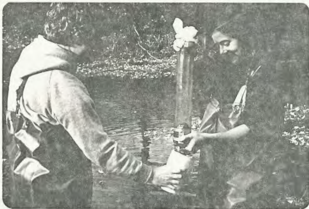
Appendix III. Core sampler used for substrate sampling in November 1980 on the Vermilion River system.
