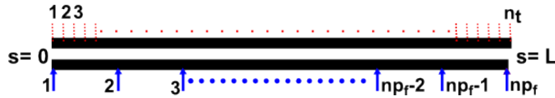
Figure 4.6: Discretization and forces acting for sensitivity calculation
