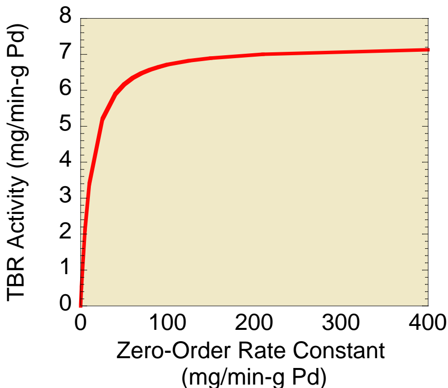
Figure 3.11: Predicted 12x30 TBR reduction activity at various intrinsic catalyst activities assuming k_{GLa} = 7.76 \text{ min}^{-1}
