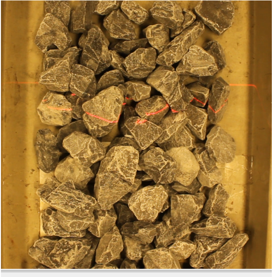
Figure 2.1: Sample Ballast Collection in Tray
