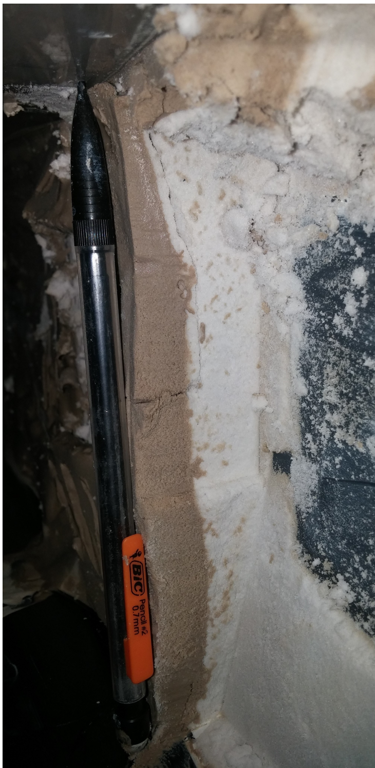
Figure 32: Photograph of deposit in section beta after one exploratory run. Image displays the contrasting deposit colors and shading due to variable kaolin content. The bare flume may be seen exposed on the bottom with the grey color.
