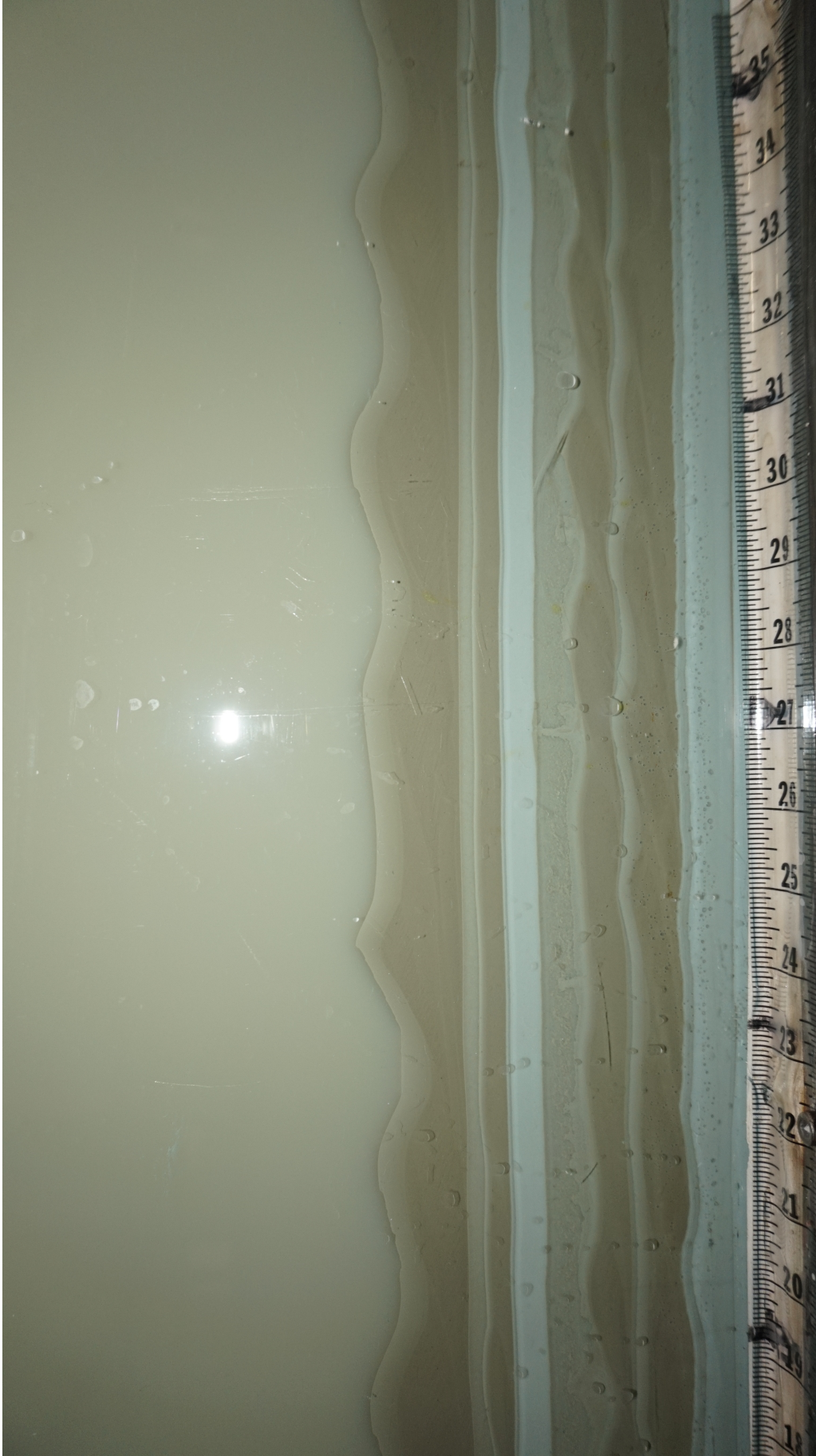
Figure 31: Photograph of deposits in section gamma after a series of seven runs. Image displays the contrasting deposit colors and shadings do to variable kaolin content. Note other features of interest including bedforms and striations.
