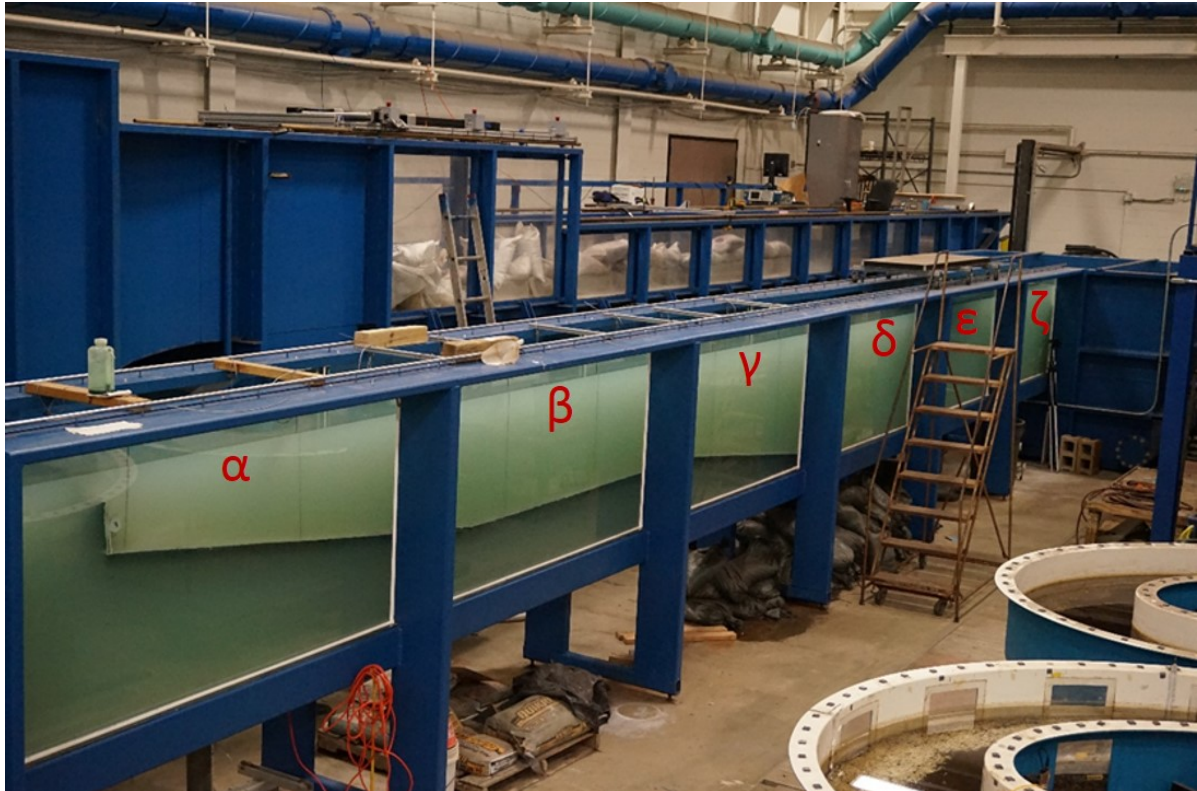
Figure 1: Photograph of the Garcia Density Current Tank at Hydosystems Laboratory, University of Illinois, used in the experiments. View is from upstream to downstream progressing from left to right and section labeling convention used in Greek letters from \alpha - \zeta . A large damping tank can be seen at the downstream end.
