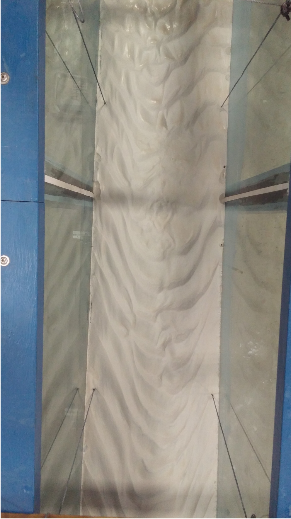
Figure 34: Plan view of 180 cm reach corresponding to sections alpha and beta (in left to right streamwise direction) of the bed after the experiment Explore 2. The slope of the bed is 7 degrees. Two-dimensional bedforms with may be seen.
