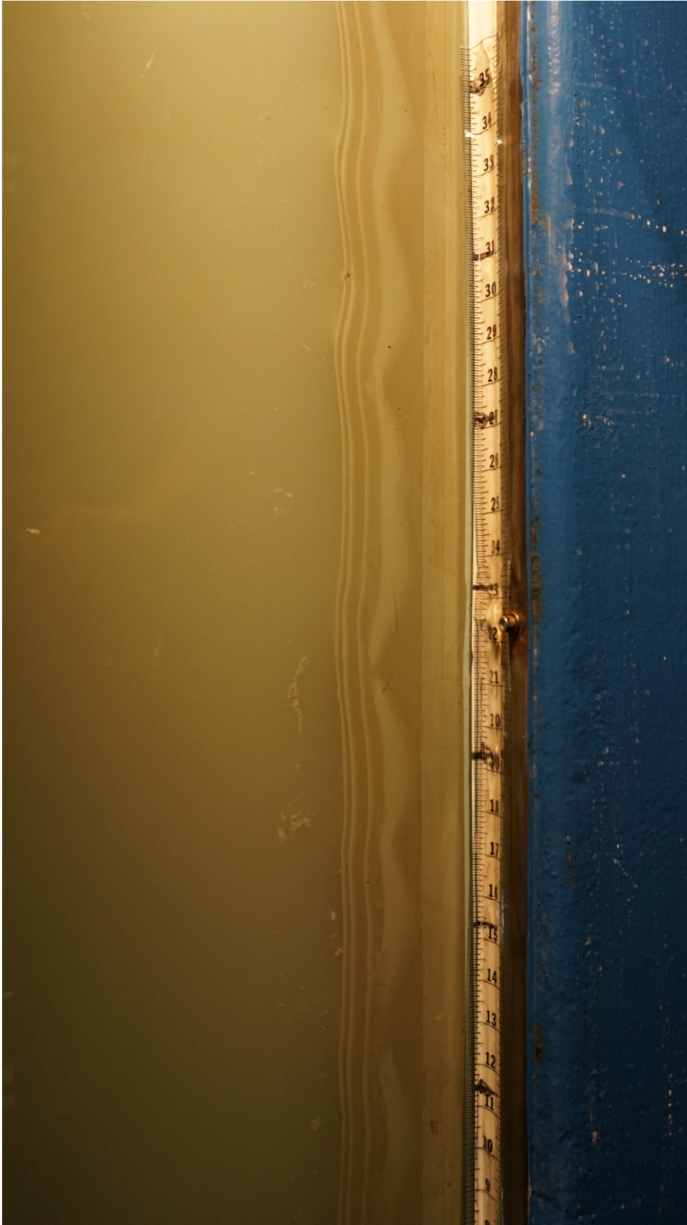
Figure 35: Profile view of 76-cm reach in section gamma with no slope and left to right streamwise direction. There are stacked deposits from runs Main 1, Bound 2, Main 2, Main 3, and Main 4 from bottom to top respectively. Bedforms from the high-concentration run Bound 2 may be seen. The darker zones correspond to relatively coarse deposits. The lighter layers are the settling caps from the very fine-grained material coming out of suspension over days.
