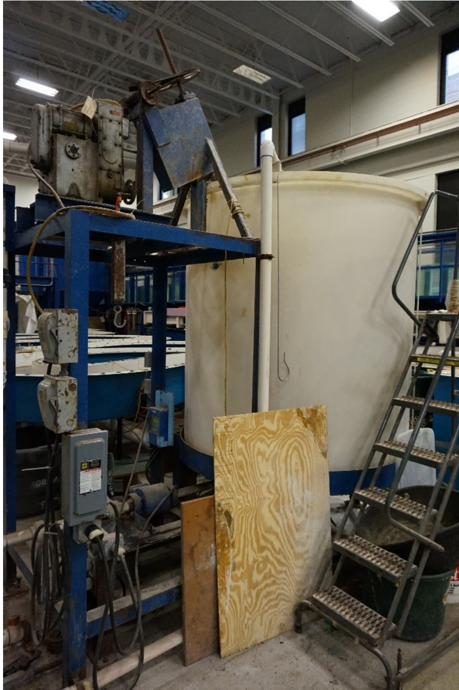
Figure 2: Mixing tank with propeller, pump setup, and piping used for creating and delivering the sediment slurries.
