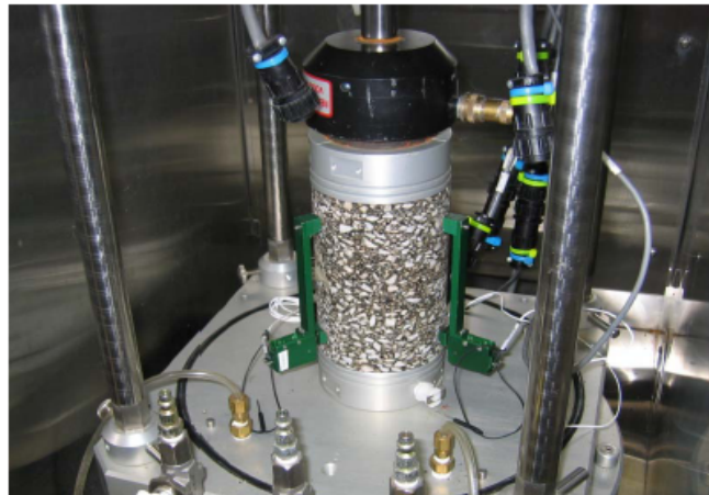
Figure 6. Complex modulus set up with three axial extensometers mounted on the asphalt mixture specimen
