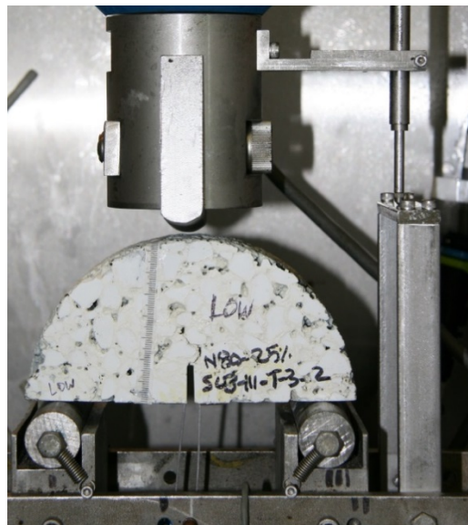
Figure 8. Semi-circular bending beam test fixture with an LVDT added for load-line displacement control
