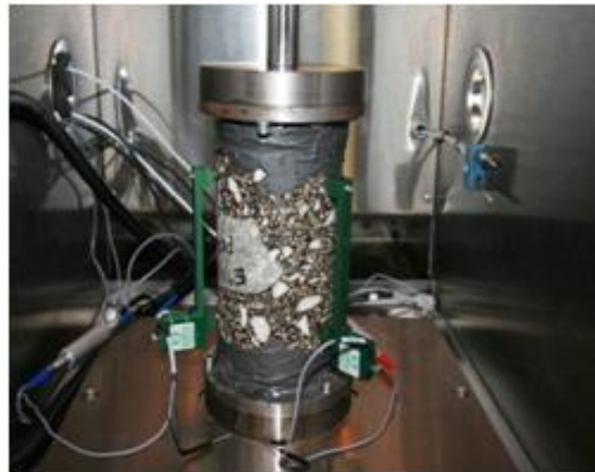
Figure 7. Push-Pull fixture setup with extensometers and specimen fixed to top and bottom plates
