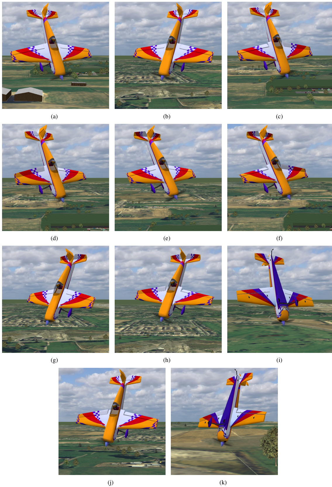
Figure 3.7: Renderings of the spins using graphics from FS One: a) T0R1E1A0-Lft-Up, b) T0R1E1A0-Rght-Up, c) T0R1E1A1-Lft-Up, d) T0R1E1A1-Lft-Up-(cross ail), e) T0R2E2A0-Lft-Up, f) T0R2E2A2-Lft-Up, g) T0R2E2A0-Rght-Up, h) T0R2E2A2-Rght-Up, i) T0R1E1A0-Rght-Inv, j) T0R1E1A1-Rght-Up, and k) T0R1E1A1-Lft-Inv.
