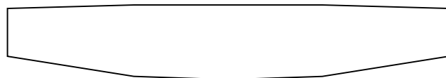
Figure 4.30: Illustration of approximate Cessna 172 wing planform as tested in this study (leading edge on top).
