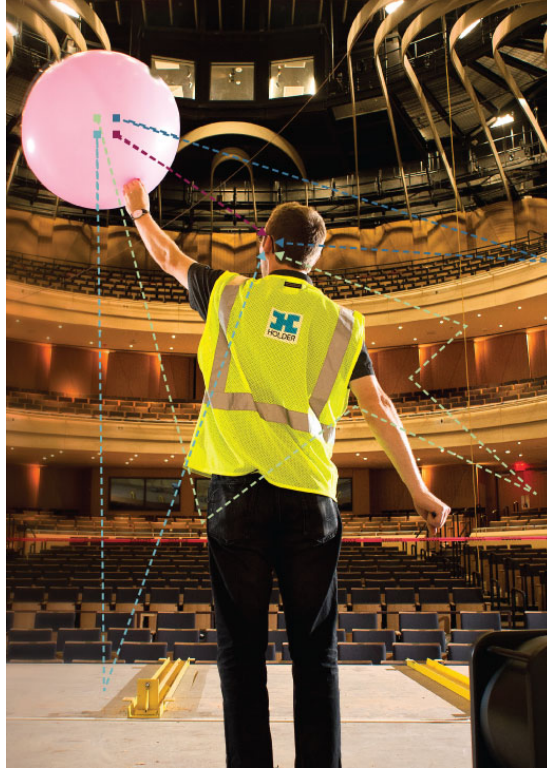
Figure 5.7: Measuring the impulse response of the Moss Art Center by popping a balloon [62].
