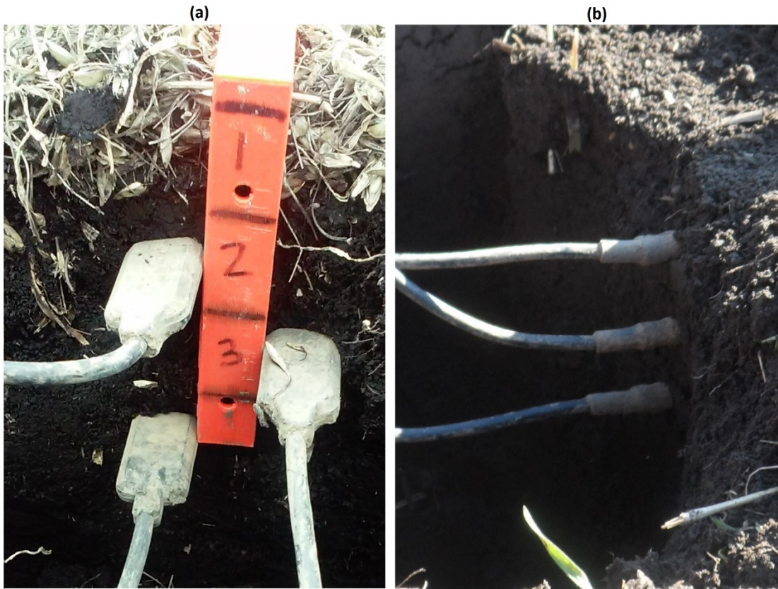
Fig. 3.4. Volumetric soil moisture contents at depths of 25, 50, and 75 mm were monitored in fields IL-11 and IL-12, while soil temperatures at depths of 25, 50, and 75 mm were monitored only in IL-12. Moisture (a) and temperature (b) sensors were inserted horizontally at each depth. Sensors were attached to data loggers and set to record every 15 minutes.
