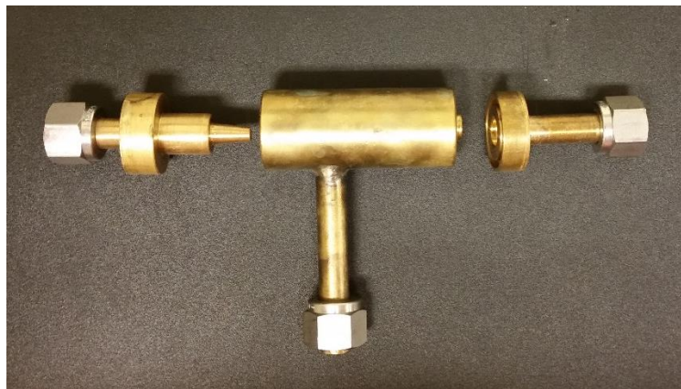
Figure 5.7: Components of modular CO 2 ejector (left to right): Motive nozzle; suction chamber and mixing section; diffuser.
