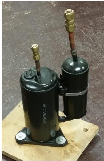
Figure C.1: Rolling-piston compressor used in R410A experimental facility.
