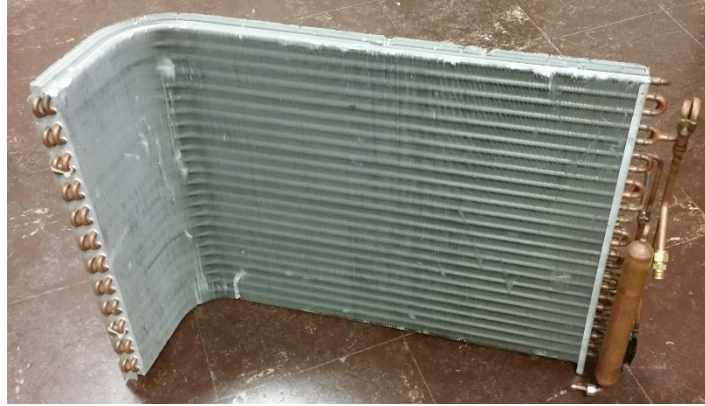
Figure C.2: Round-tube-plate-fin condenser used in R410A experimental facility.
