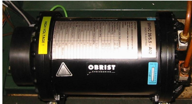
Figure C.3: Semi-hermetic, reciprocating compressor used in CO 2 experimental facility.
