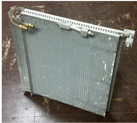
Figure C.5: Microchannel gas cooler/condenser used in CO 2 experimental facility.
