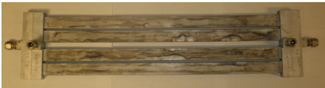
Figure C.6: Microchannel internal heat exchanger used in CO 2 experimental facility.
