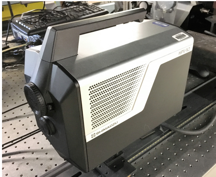
Figure 2.9: Image of the Shimadzu HPV-X2 camera used for the high-speed shadowgraph images obtained in T5.
