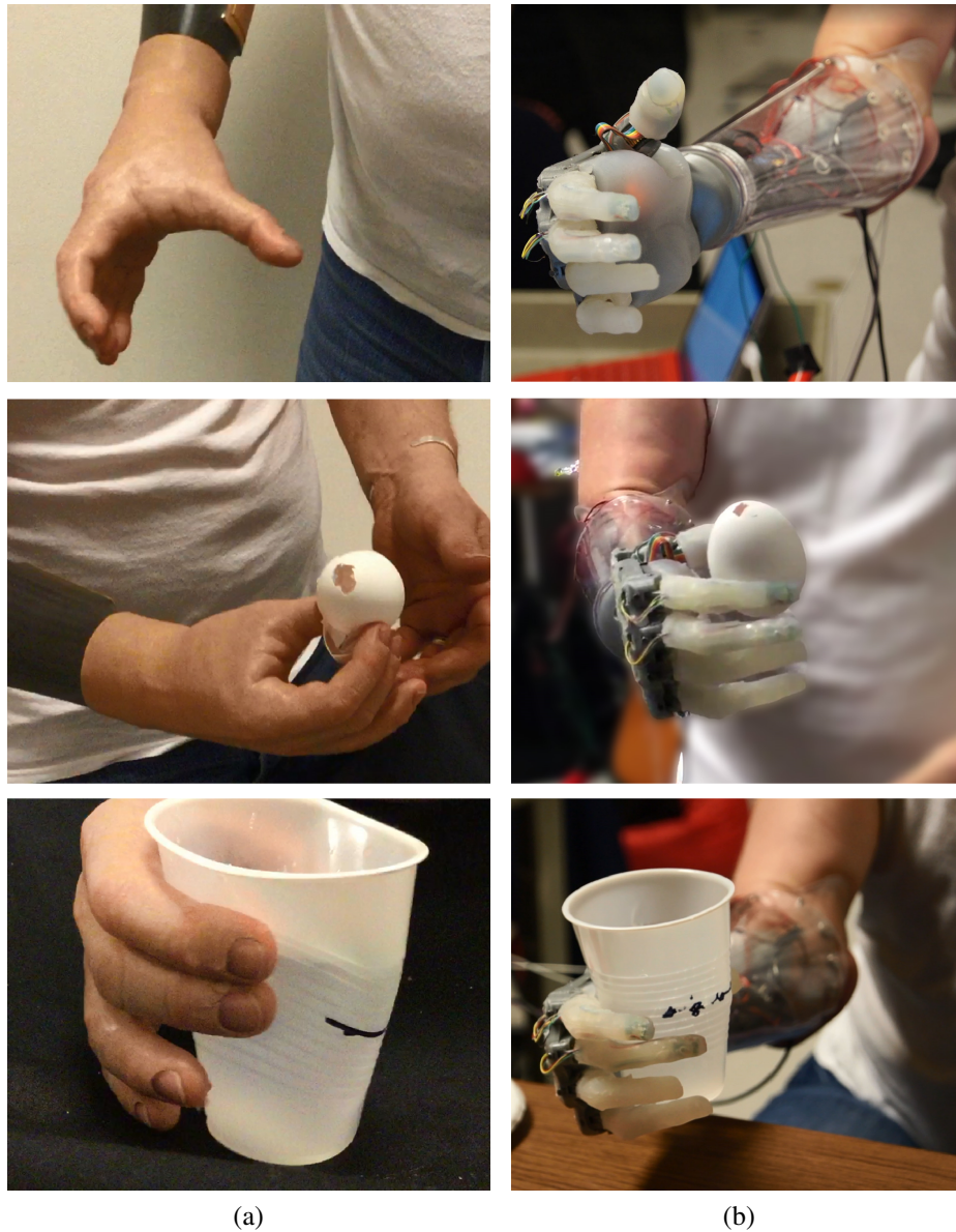
Figure 4.6: Experiments with (a) the subject's original myoelectric prosthesis showing him crushing the egg and cup. However, when using the new hand as shown in (b), he successfully grasps the egg without cracking it and grips the cup with minimal water displacement.
