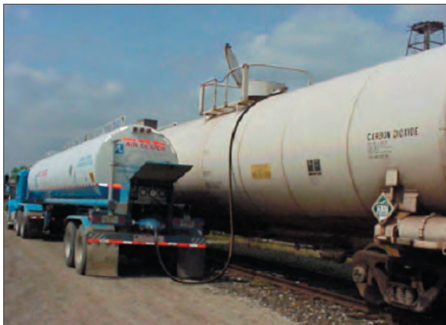
Figure 4.2. Unloading CO 2 from railcar to truck
