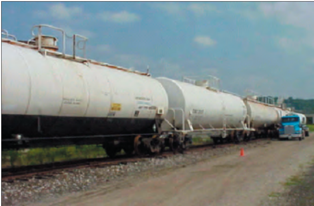
Figure 4.1. Typical CO 2 railcar
