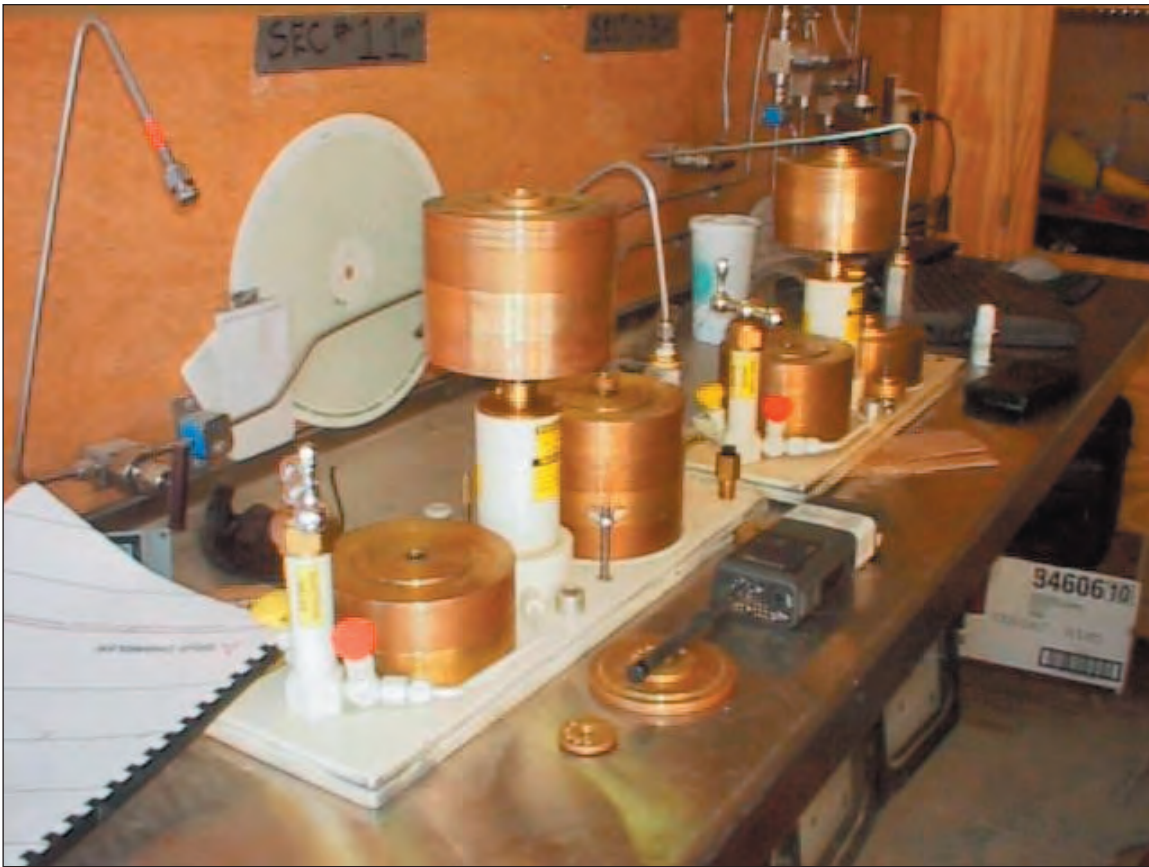
Figure C1.35. Hydrotest pressures provide accurate measurement using dead weight and testers
