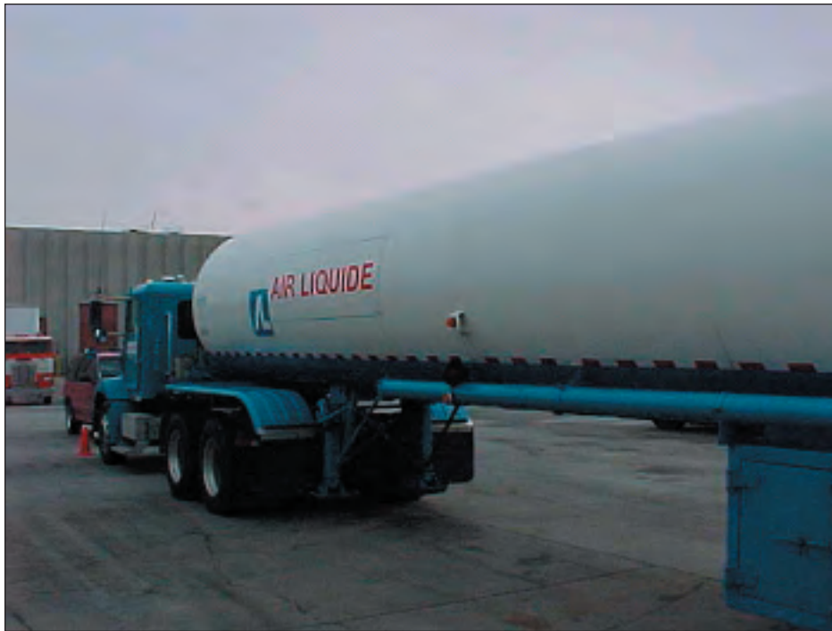
Figure 3.1. Typical CO 2 truck trailer
