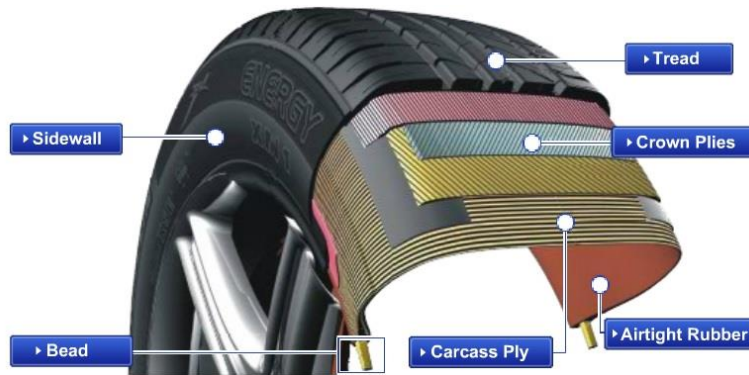
Figure 1-1. Schematic representation of tire basics (from Michelin website on November 6 th 2014).
