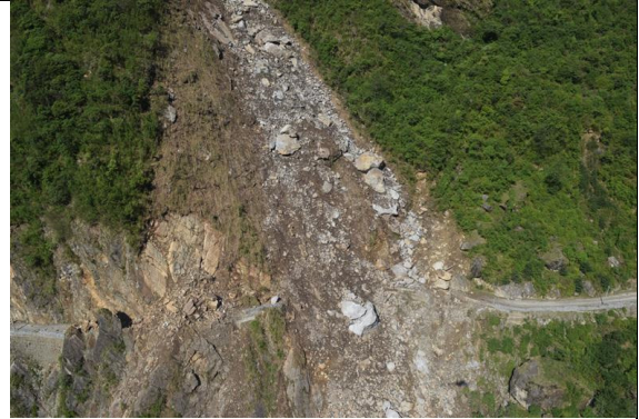
Figure 2.10 Large scale landslides that affected the Charikot-Lamabagar Road sector.
