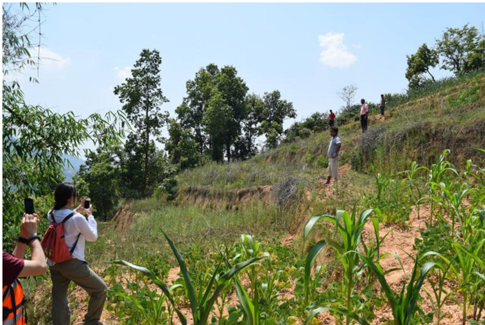
Figure 2.6 Head scarp observed on the ridge of the slope triggered by the 2015 earthquake (after Hashash et al. 2015).
