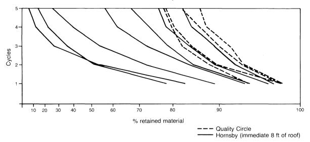
**Figure 23** Slake durability results for Energy Shale from the Hornsby district and the Quality Circle. All samples within 8 ft (2.4 m) of the top of the Herrin Coal. From Robert A. Bauer.
