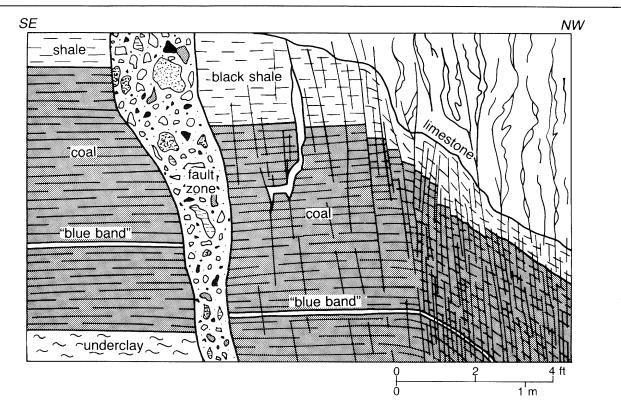
**Figure 20** Field sketch of part of strike-slip fault zone in Crown II Mine. The wide vertical fissure (left of center) contains a loosely packed jumble of coal, shale, limestone, and sandstone fragments. To the right, coal and roof are shattered by hundreds of vertical fractures, many of them open. Fissures and open fractures yield large amounts of water.
