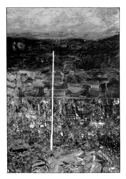
**Figure 10** Anna Shale overlain by smooth-bottomed Brereton Limestone. Lower half of Anna is hard, fissile, and well jointed; upper half is less competent and more massive. Ruler measures 4 feet (1.2 m).
