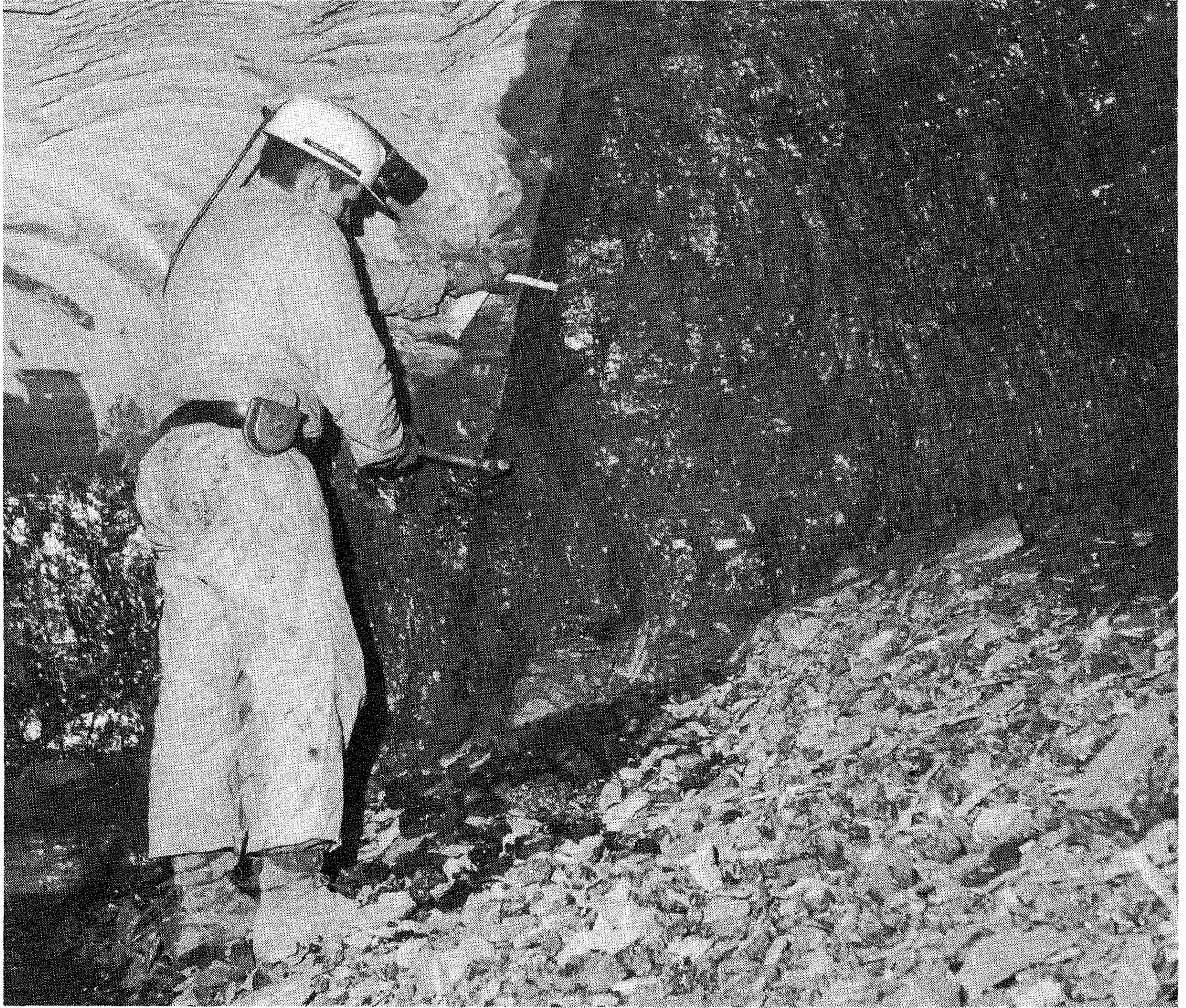
A typical fault of the Rend Lake Fault System exposed in the Orient No. 6 Mine. The Herrin (No. 6) Coal is offset about 6 feet; this necessitates mining the rock to maintain grade. Features to note include: steep angle of fault plane, absence of drag, and narrow zone of gouge. Photo by Heinz Damberger.
