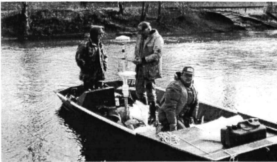
Figure 15a. Reconnaissance survey crew preparing to depart for the day's work. Field equipment includes RTCM corrected GPS and maps
