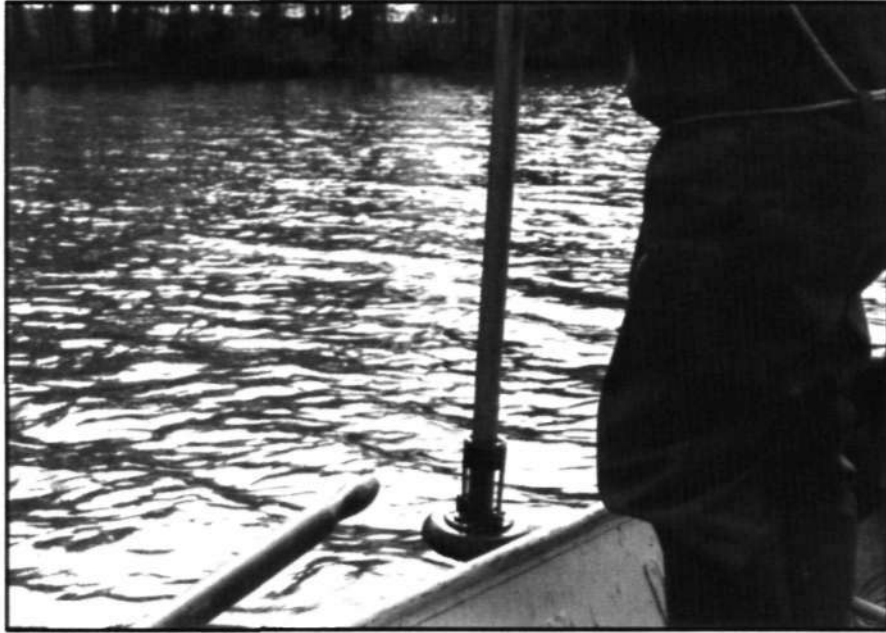
Figure 9. Sounding pole fitted with sliding shoe
