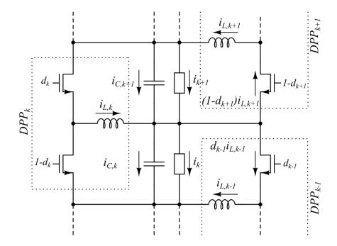
Figure 2.6: A single DPP converter with adjacent converter elements
