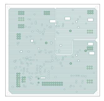
Figure A.14: Hysteretic control board for DPP layout, layer 2 (gnd planes)
