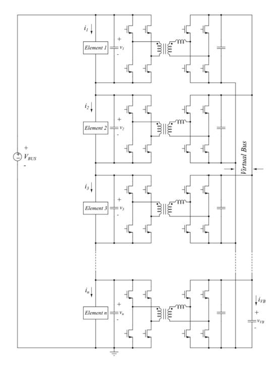
Figure 2.3: Virtual bus-to-element topology using full bridge isolated converters as DPP converters
