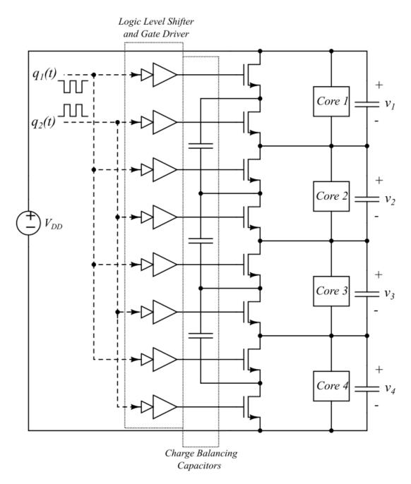
Figure 2.5: Switched capacitor voltage balancing circuit
