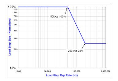
Figure 1.10: Transient repetition rate [5]
