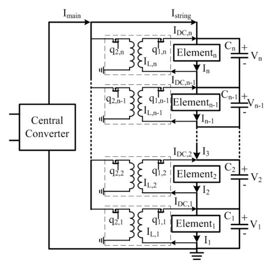
Figure 2.2: Series connected bus-to-element DPP using n isolated flyback converters [25]
