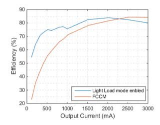
Figure 5.3: Individual DPP converter efficiency plot in FCCM and with light-load mode enabled,  $L = 1 \ \mu\text{H}$ ,  $f_{sw} = 500 \text{ kHz}$
