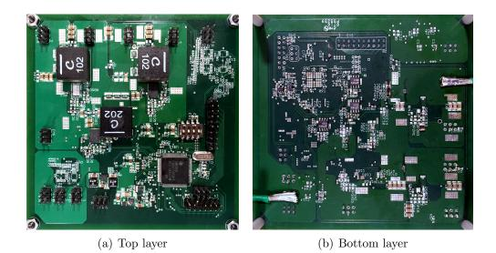
Figure 5.2: DPP board with 3 converters
