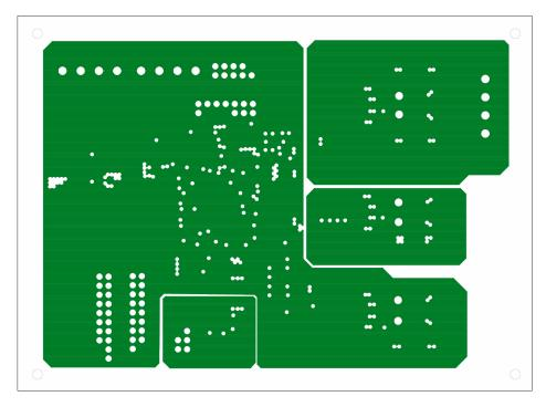
Figure A.6: Linear control board for DPP layout, layer 2 (gnd planes)
