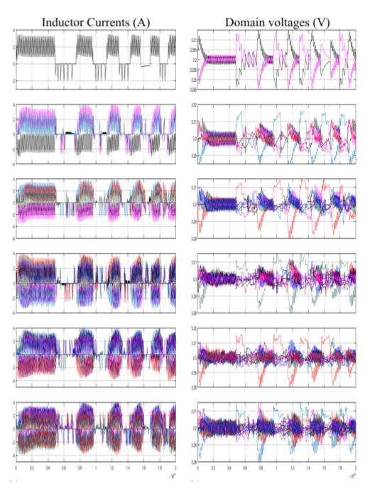
Figure 4.17: Transient responses to a step in mismatch current for a current hysteretis controlled stack - bidirectional light-load modes enabled; number of stacked elements increases from top to bottom (2 at top, 12 at the bottom)
