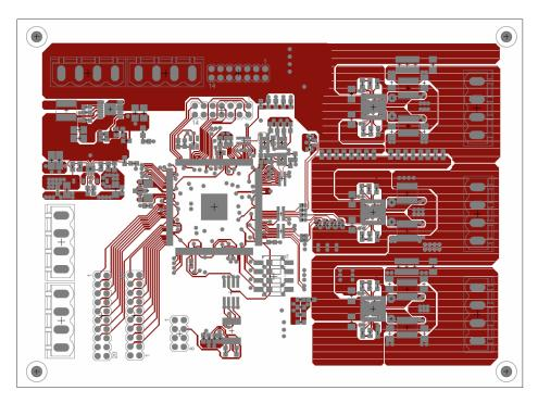
Figure A.4: Linear control board for DPP layout, top layer
