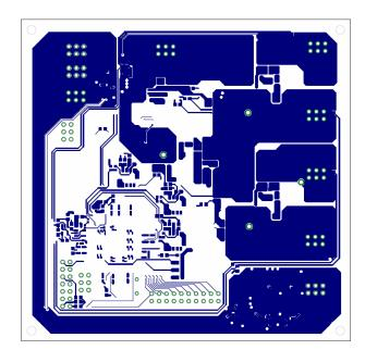
Figure A.13: Hysteretic control board for DPP layout, bottom layer
