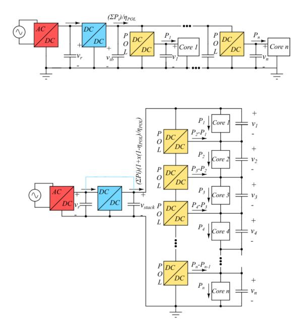
Figure 1.13: IBA vs. series-connected power delivery: The architecture shown at the top is the integrated bus architecture (IBA) and the lower one is a high level diagram of the series-connected power delivery architecture.
