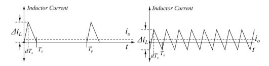
Figure 4.1: Single pulse PFM mode (left) and FCCM mode (right) inductor currents at same average output current
