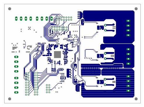
Figure A.5: Linear control board for DPP layout, bottom layer
