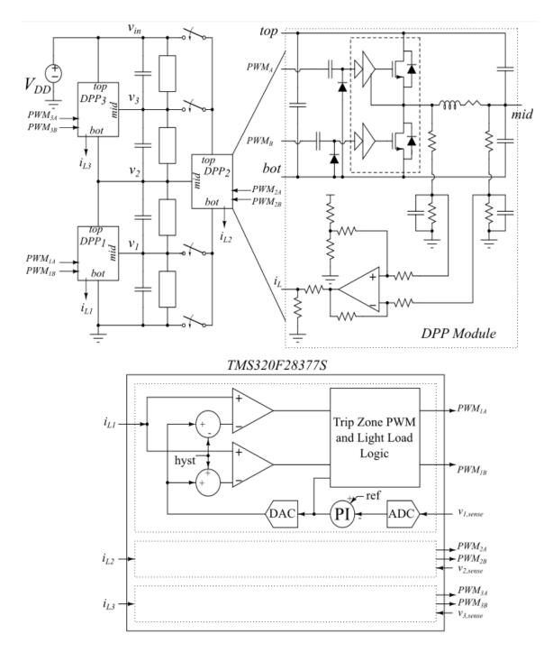
Figure 5.1: Hysteretic current mode control hardware setup
