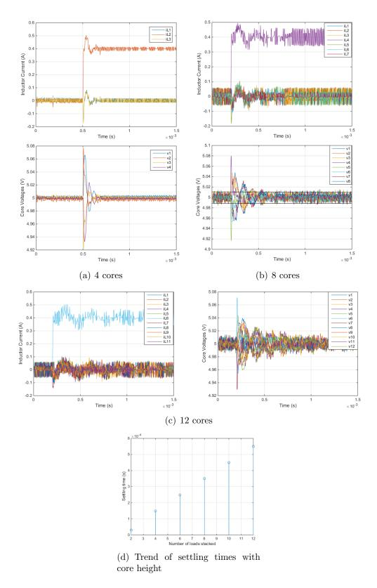
Figure 2.11: Simulated trend in settling times with increasing number of series-stacked elements
