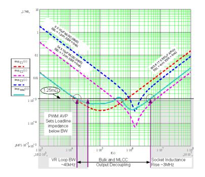
Figure 1.6: Typical impedance of a composite system of capacitors (bulk electrolytic, MLCC decoupling and MLCC cavity capacitors) - [5]
