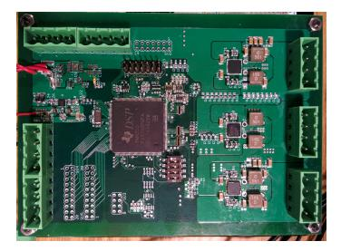
Figure 3.2: DPP board with 3 converters
