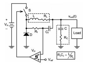
Figure 4.6: Droop control of hysteretic buck converter
