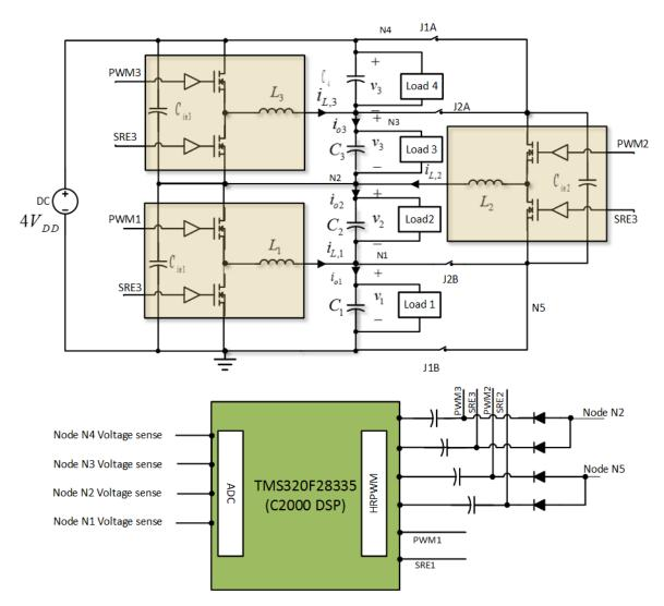
Figure 3.1: High-level schematic of the implemented hardware
