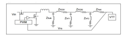
Figure 1.5: Typical buck converter output filter structure with parasitic components [5]
