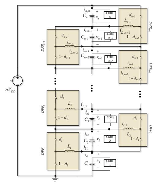
Figure 2.4: Element-to-element topology
