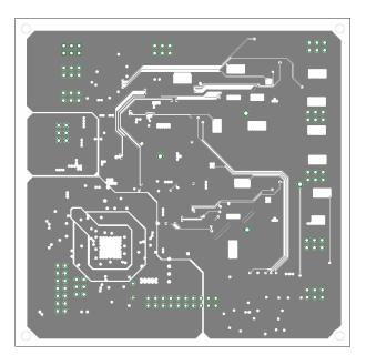
Figure A.15: Hysteretic control board for DPP layout, layer 3 (microcontroller supply)
