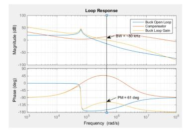
Figure 1.3: Compensation of buck converter
