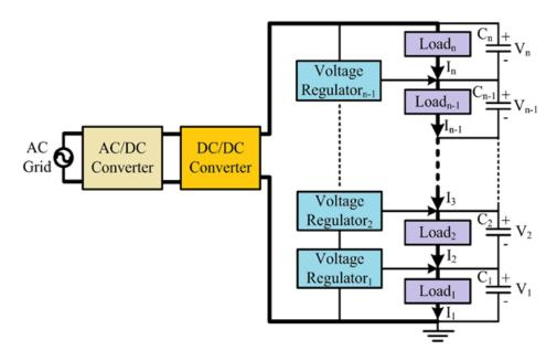
Figure 1.12: Series-connected power delivery
