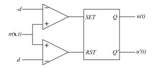
Figure 4.2: Sliding mode switching signal generation
