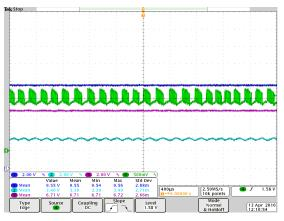
(a) Lowermost converter operating in DCM, green: sensed inductor current of the lowermost converter
