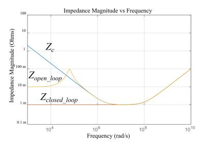
Figure 1.4: Open loop and closed loop output impedance of buck converter under droop control
