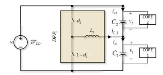
Figure 2.8: DPP converter module
