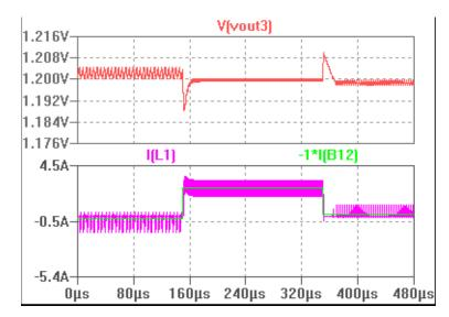
Figure 4.9: Hysteretic control with load current sensing
