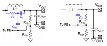
(a) Current ripple feedforward (b) Voltage ripple feedforward
