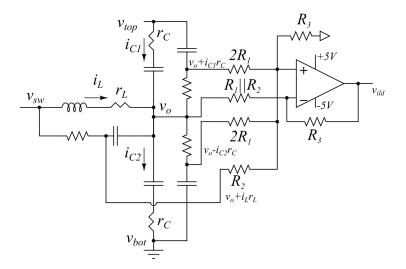
Figure 4.8: Load current estimation of DPP converters
