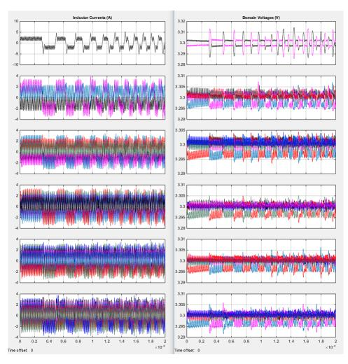
Figure 4.15: Current hysteretis controlled stack - high static gain current estimator; number of stacked elements increases from top to bottom (2 at top, 12 at the bottom)
