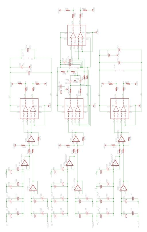
Figure A.11: Hysteretic control board for DPP schematic, microcontroller supply
