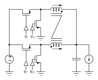
Figure 1.11: Coupled inductor 2-phase buck converter
