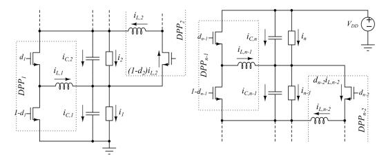
Figure 2.7: DPP converters at the extremities of the stack
