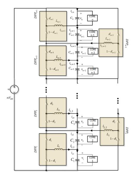
Figure 2.12: Hierarchical element-to-element DPP
