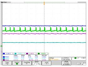
(b) Topmost converter in negative DCM and converter at the middle of the stack in DCM, green: sensed inductor current of the latter
