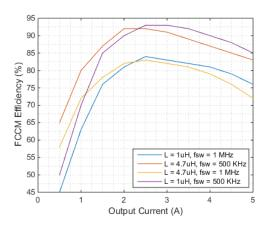
Figure 3.8: Individual DPP converter efficiency plot
