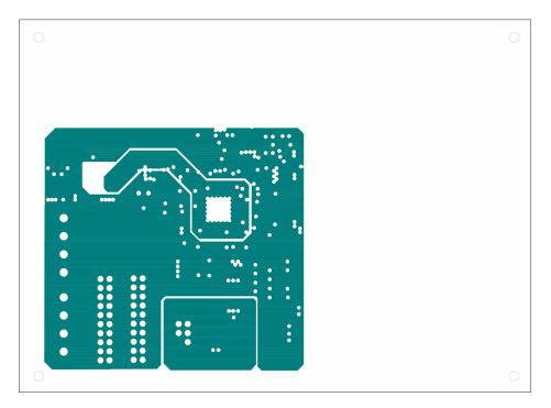
Figure A.7: Linear control board for DPP layout, layer 3 (microcontroller supply)
