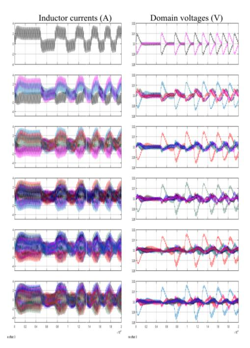
Figure 4.16: Transient responses to a step in mismatch current for a current hysteretis controlled stack in FCCM - PI controller in current estimator; number of stacked elements increases from top to bottom (2 at top, 12 at the bottom)
