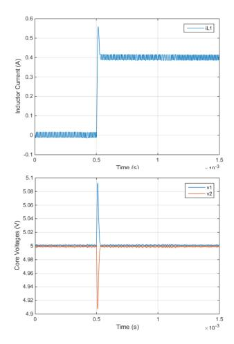
Figure 2.10: Load current step response, 2-core case
