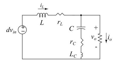
Figure 1.2: Buck converter averaged model
