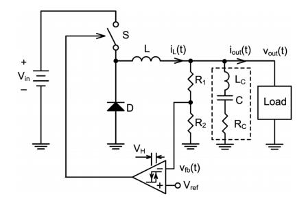
Figure 4.3: A buck converter with hysteretic control
