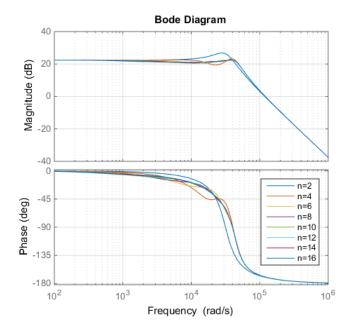
Figure 2.9: Frequency response of converters at the middle of the stack. n = stack height
