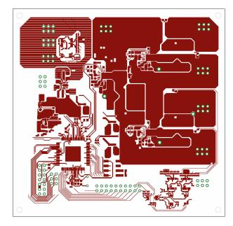
Figure A.12: Hysteretic control board for DPP layout, top layer
