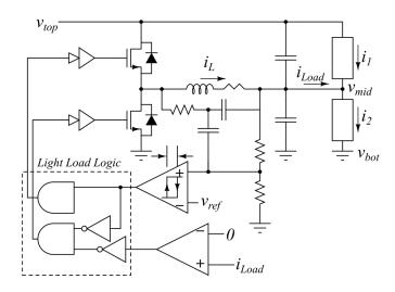
Figure 4.7: Bidirectional DPP converter with hysteretic control
