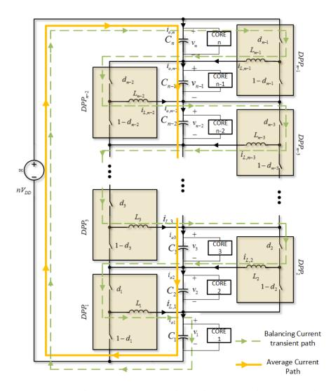
Figure 2.13: Balancing current path in element-to-element topology
